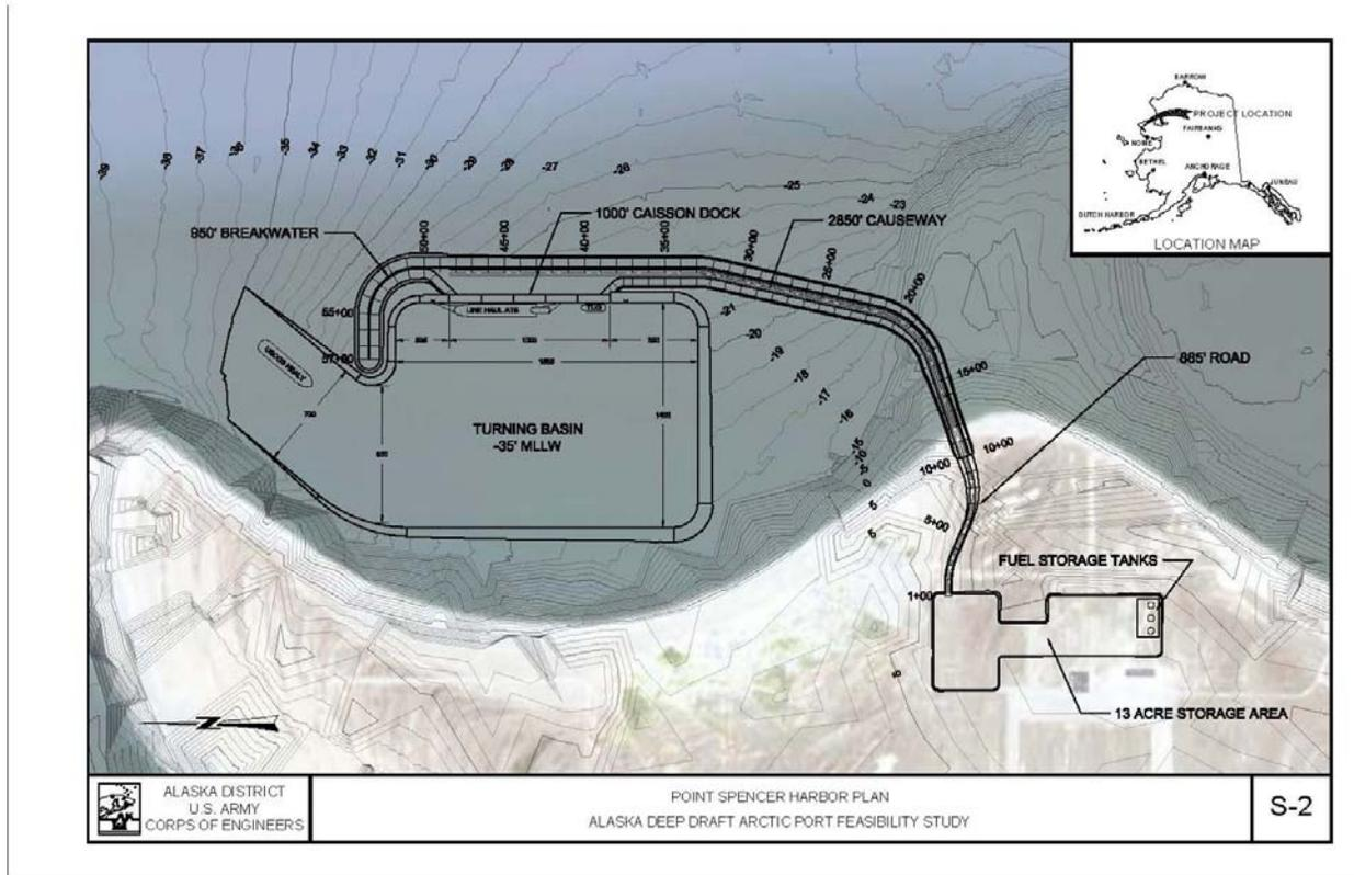
Figure 2.3. Preliminary Point Spencer layout. Source USACE (2013).
