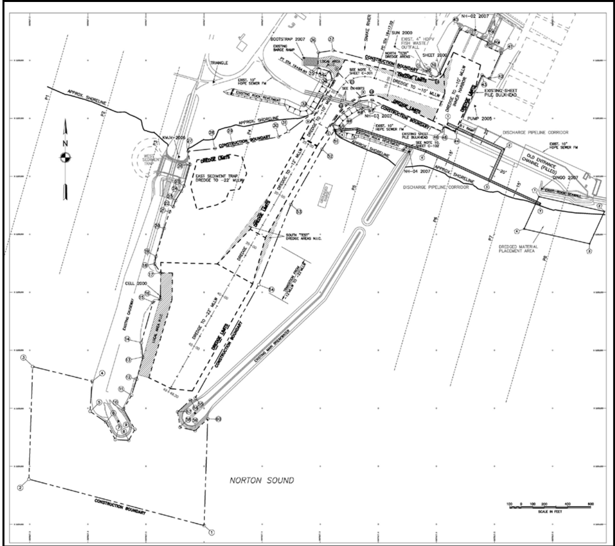
Figure 2. Drawing of proposed limits of dredging, and the dredged material placement area (excerpted from USACE 2012).
