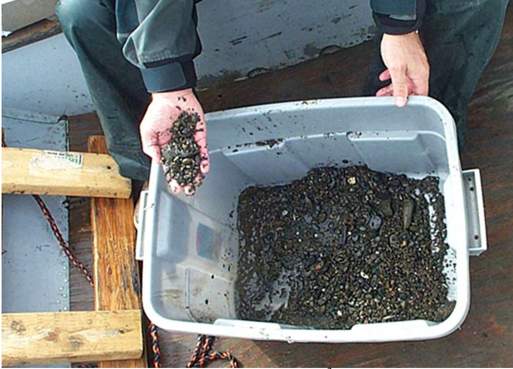
Example of benthic material collected using a 1m 3 dredge.
