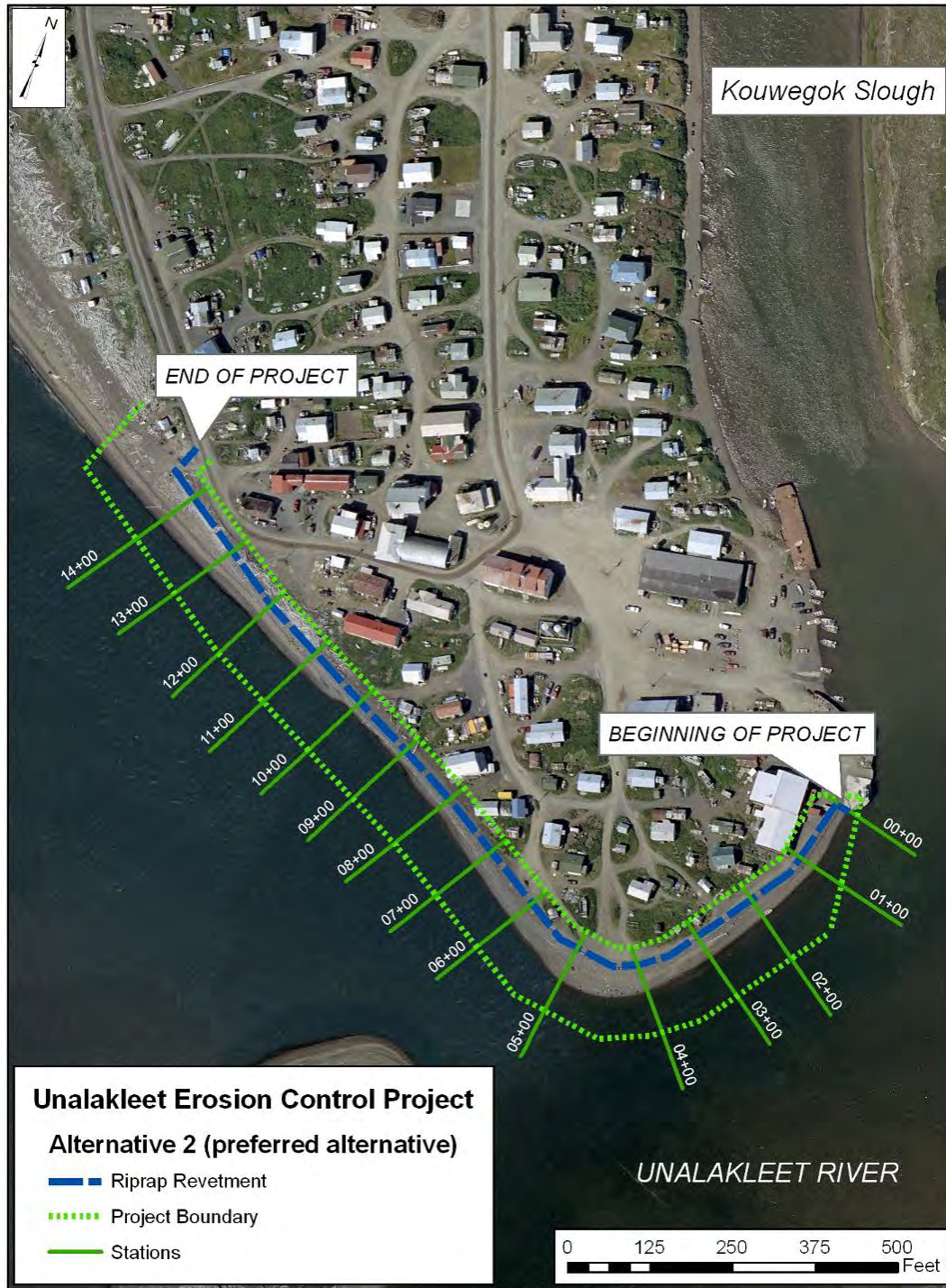
Fig. 2. Location of proposed Alternative 2-Riprap revetment.
