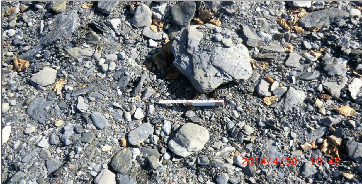
Figure 3: Typical alluvial deposits including boulders, cobbles, and gravel used in the construction of the existing berm.
