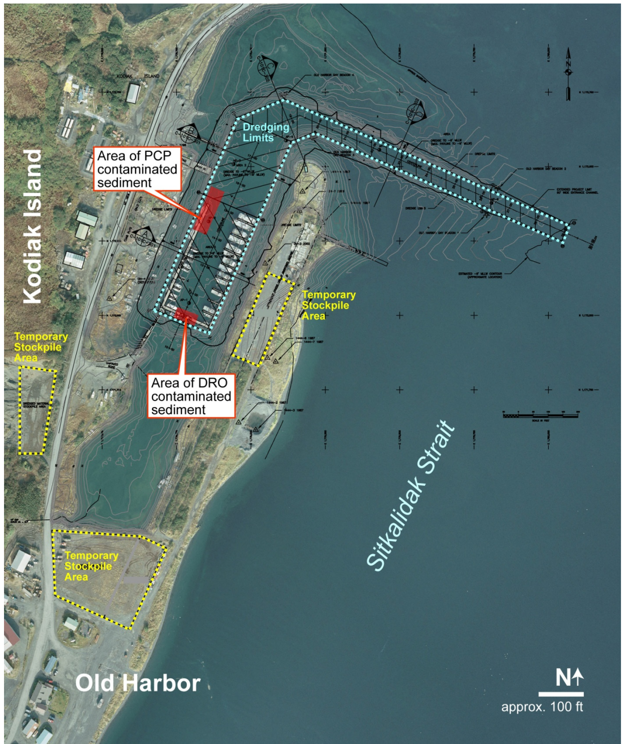
Figure A-2. Layout of harbor dredging limits, and proposed dredged material handling areas.
