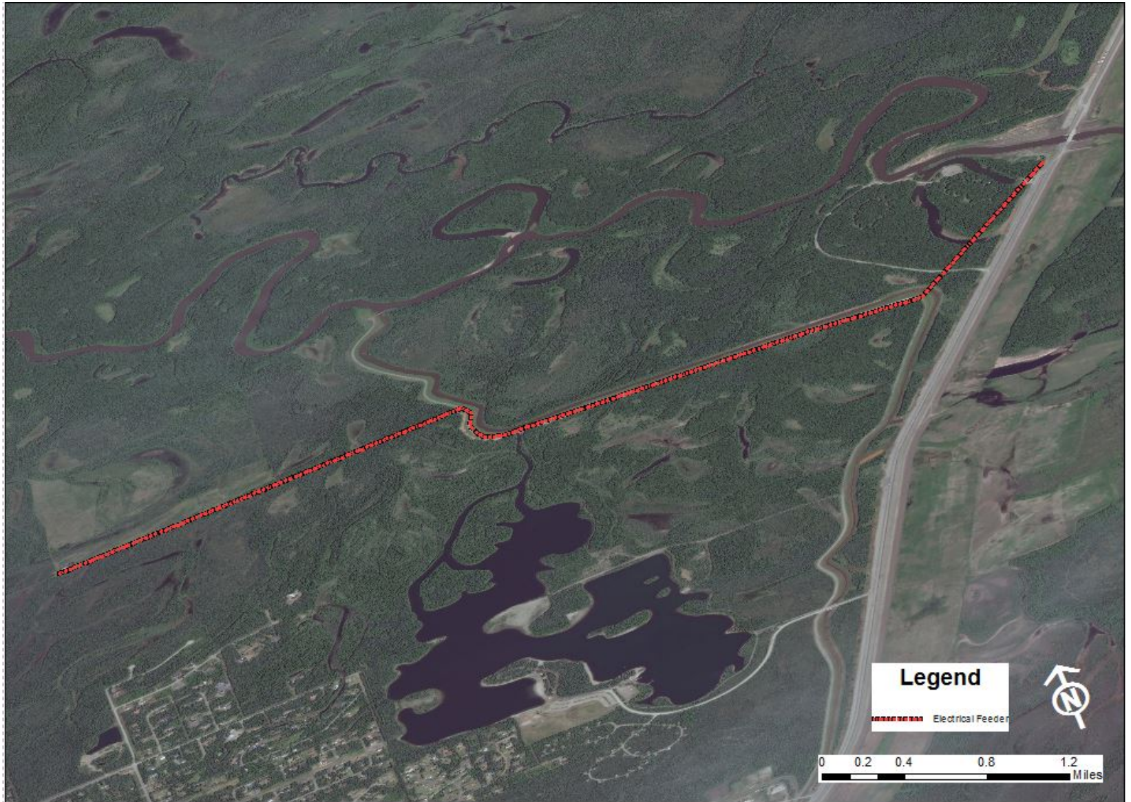
Figure 2. Proposed electrical feeder alignment
