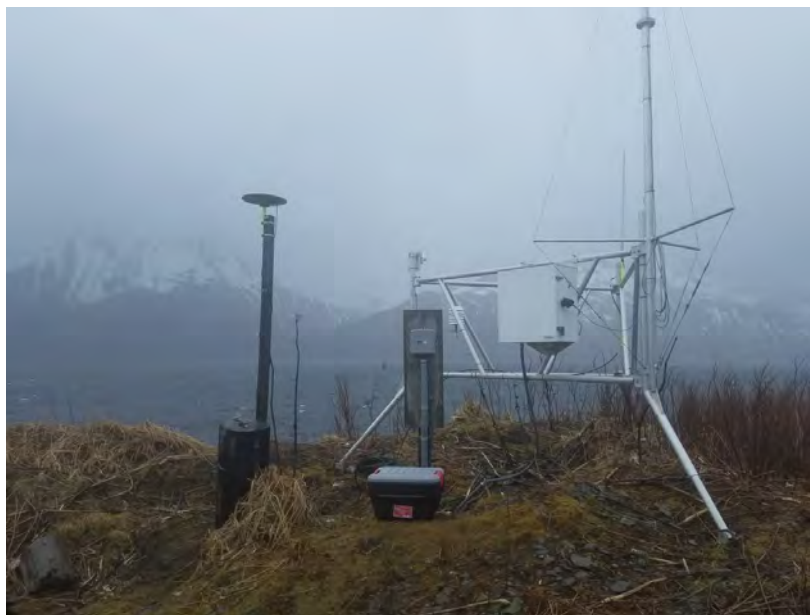
Figure 7 Trimble SP 855 RTK base station "SPIT" GNSS & VHF Antennas set-up for the project
