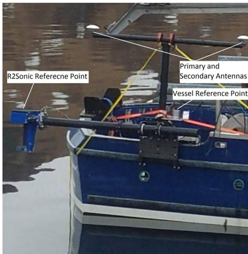
Figure 5 Vessel Central Reference Point
