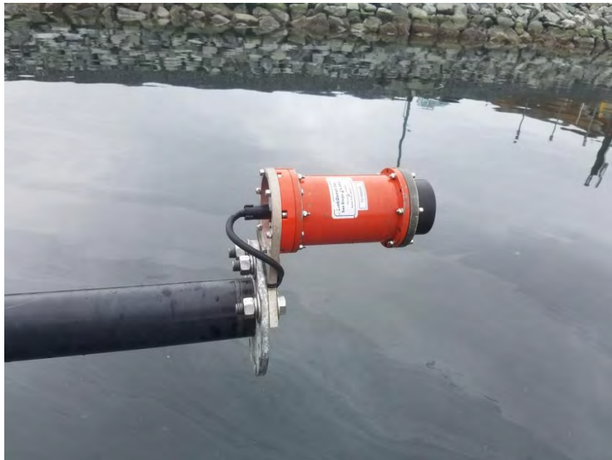
Figure 25 USBL Mounted on end of VOOP USM
