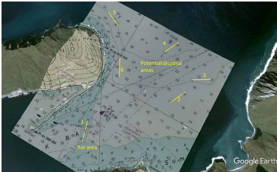
Figure 6. Potential Dredged Material Placement Areas
