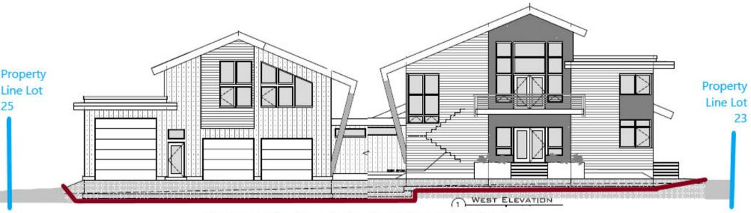
Graded and filled area depicted on flattened West Elevation Excavation of as much as 5' in the north (left) corner and as little as 1.5' to the south (rt)
