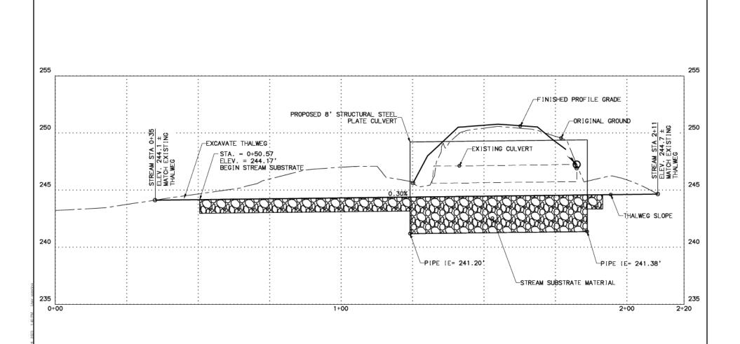
FIGURE 3a: Elevation View - Proposed Culvert POA-2023-00148
