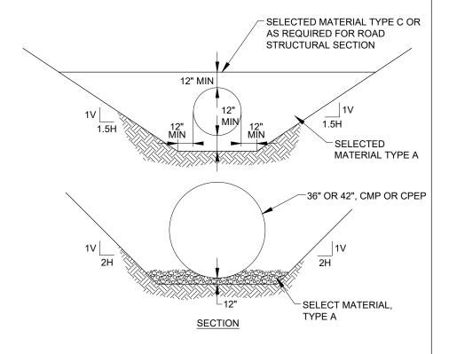
TYPICAL CULVERT CROSS SECTION AT SEWARD HIGHWAY
