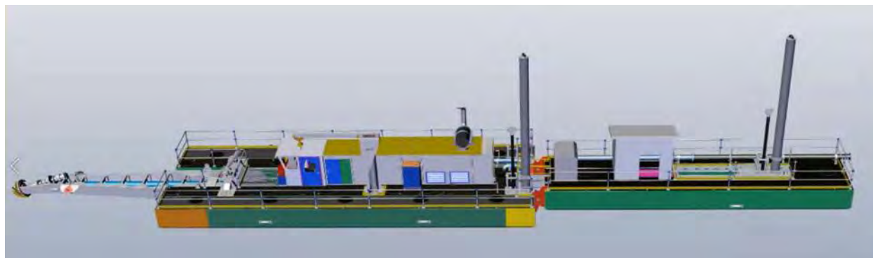
Figure 5-10. Complete assembled cutterhead dredge and idler float
