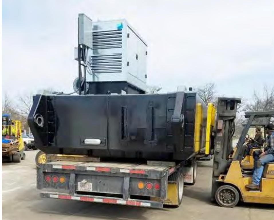
Figure 5-9. Idler float showing pin bushings where it attaches to the dredge
