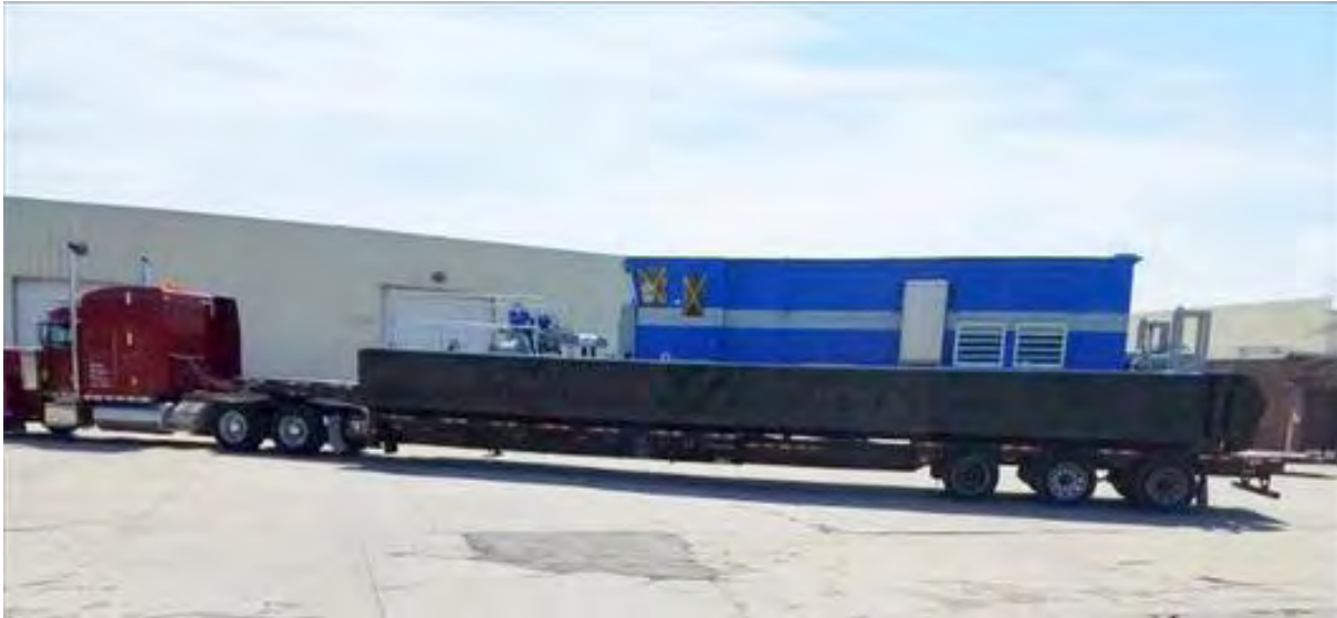
Figure 5-6. Front section of dredge barge on a trailer
