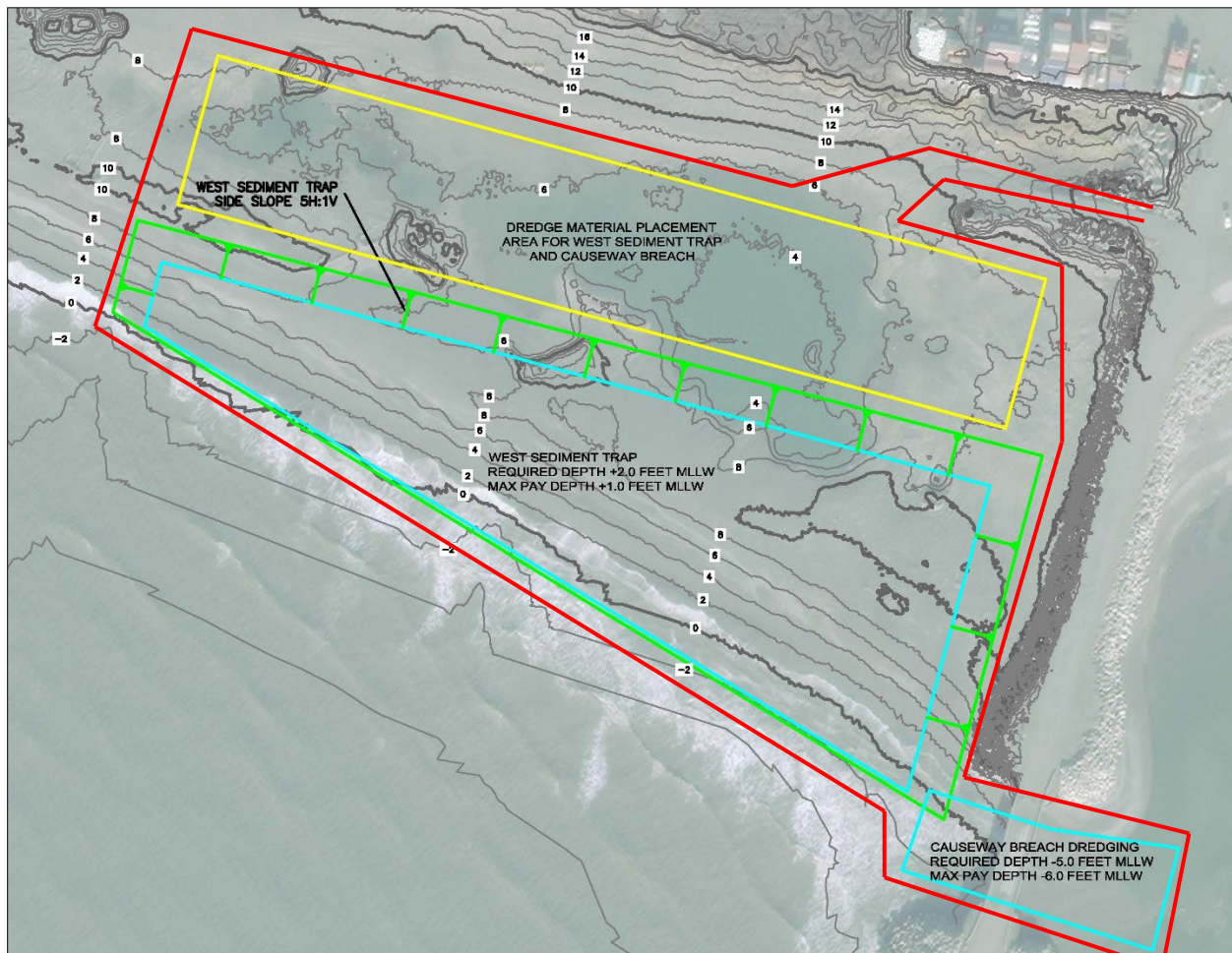
9. Proposed new dredging and disposal area along the west beach, Nome Harbor. Project APE in red, dredging area in green and blue, disposal area in yellow.
