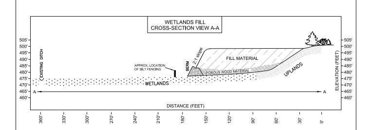
WITHIN THIS OVERALL SCOPE OF THIS PROJECT PLACE APPROX. 12,000 C.Y. OF WOODY DEBRIS, 75,000 C.Y. OF OVERBURDEN AND 12,000 C.Y. OF PEAT/TOP SOIL IN APPROX. 1.97 ACRES OF KETTLE AND DISCHARGE SLOPE WETLANDS FOR A PERMITTED FILL SITE FOR UNUSEABLE CONSTRUCTION MATERIAL. INSTALL APPROX. 40' CMP UNDER A 30' WIDE BASE FOR ACCESS ROAD.
