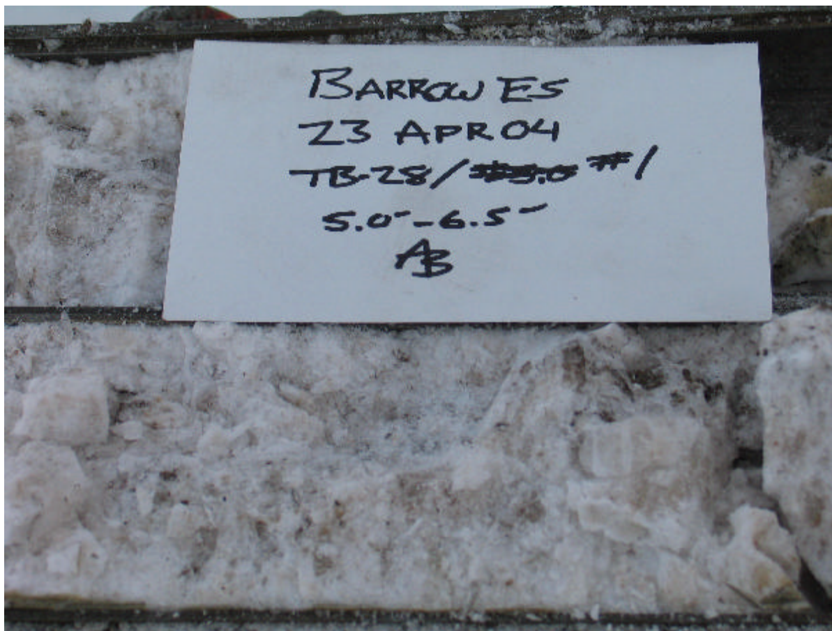
Photo 6. Example of a high ice content sample from the BIA Prospect.
