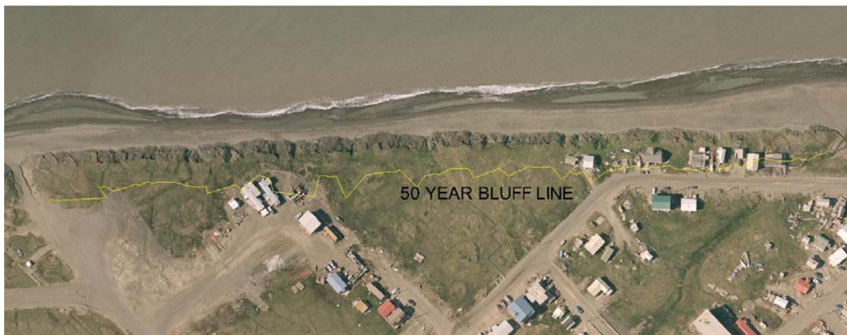
Figure 70. Location of bluff line in 50 years using the average erosion rate, not the “hot spot” rate.
