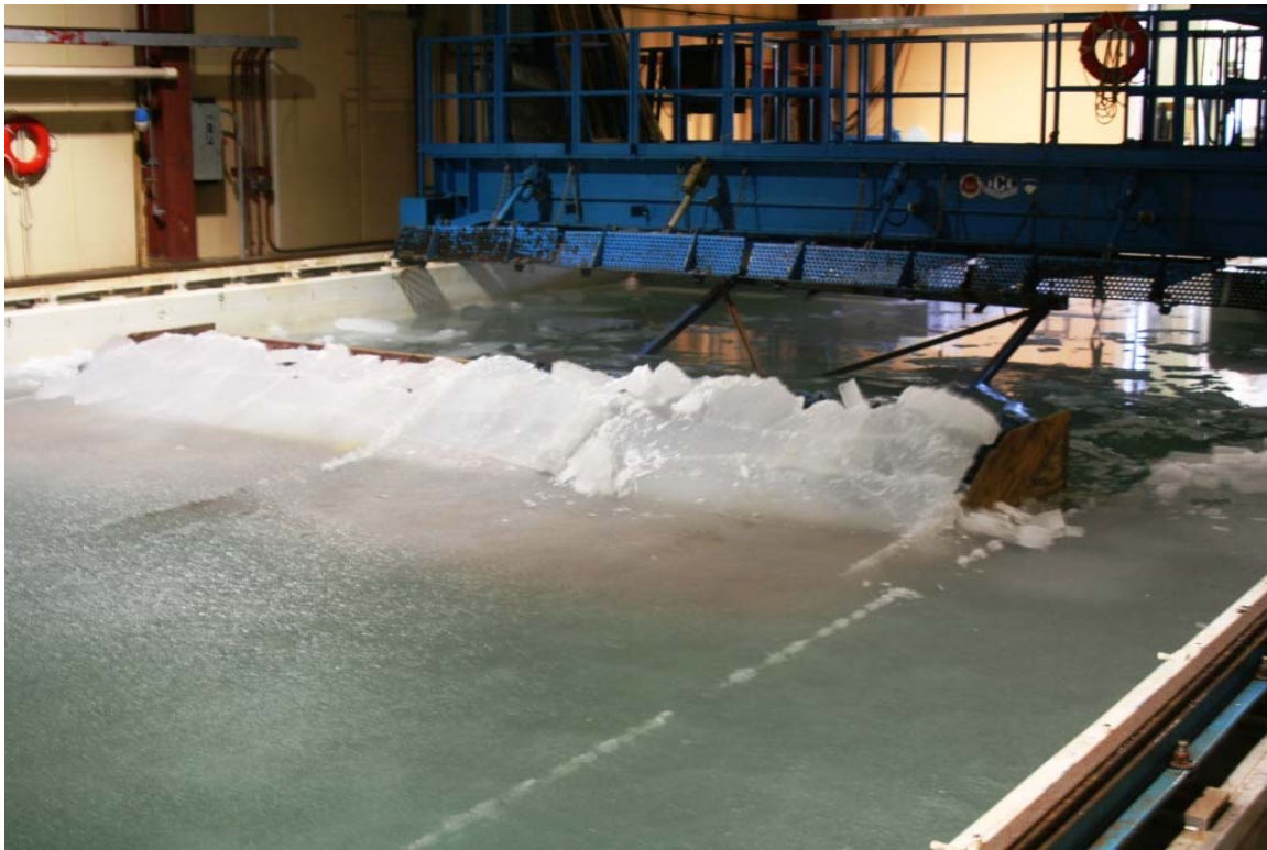
Figure 103. Revetment test section being pushed by carriage.
