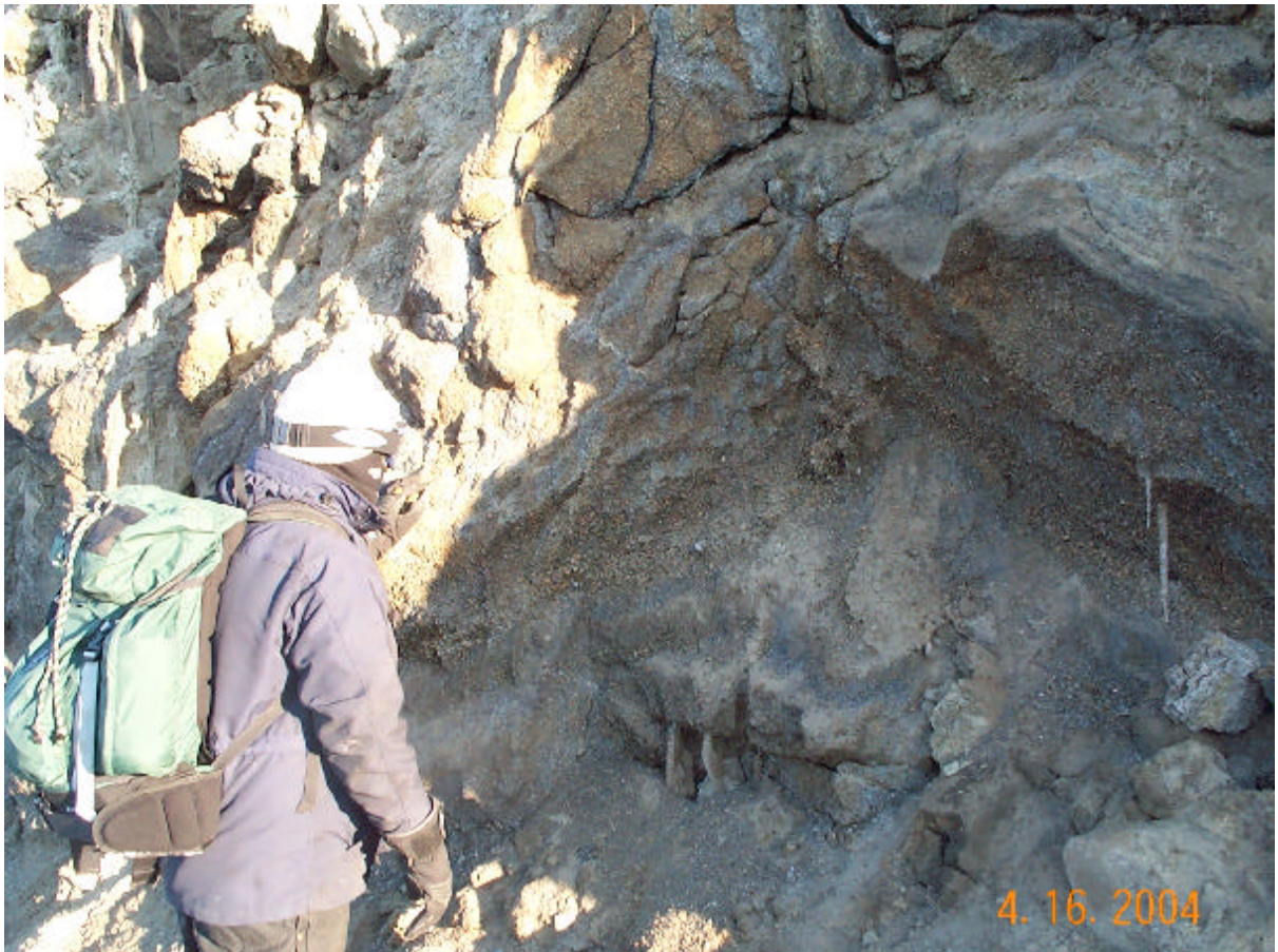
Photo 8. Typical "gravel" deposit in sidewall of existing borrow area.
