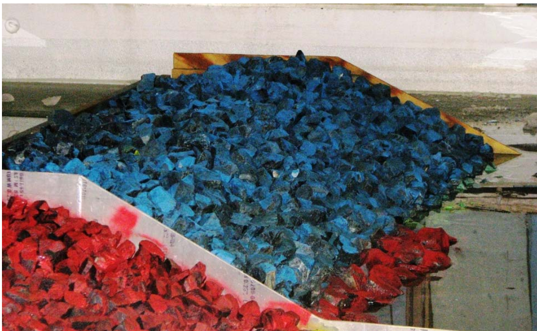
Figure 105. 8-ton armor stone (blue slope) with 13-ton toe (red toe stone) revetment before ice testing.
