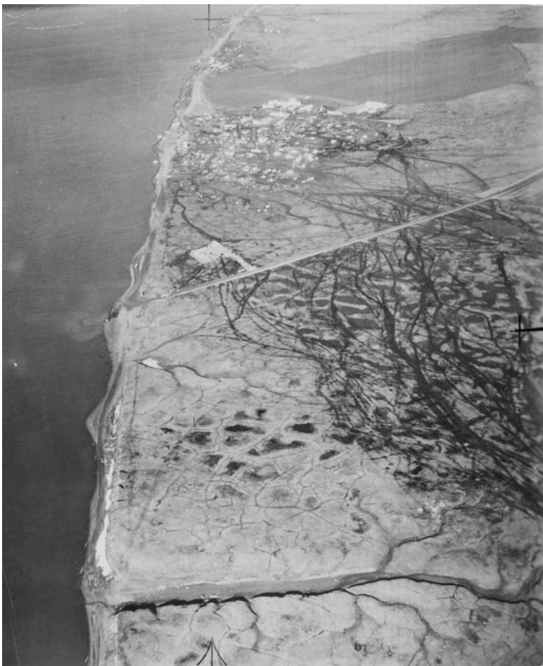
Figure 75. Scalped shoreline consistent with beach borrowing.
