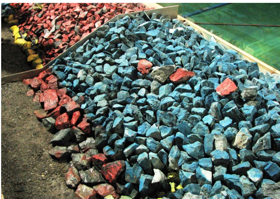
Figure 106. 8-ton armor stone (blue slope) with 13-ton toe (red toe) stone revetment after ice testing. Some toe stone moved during test, but the revetment slope stayed intact.
