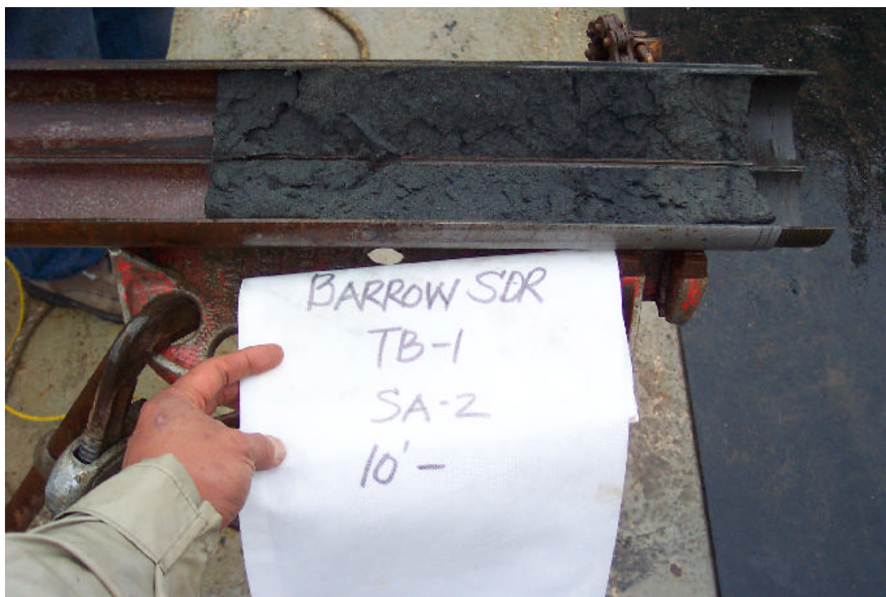
Photo 10. Typical sand encountered during the drilling operation.
