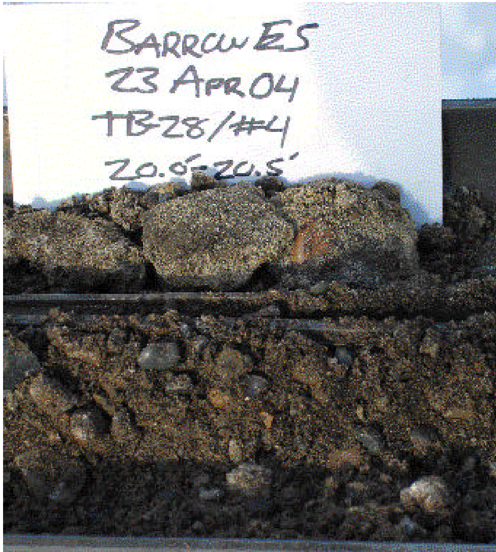
Photo 9. Typical Poorly Graded Sand with Gravel (SP) encountered on the BIA Prospect.
