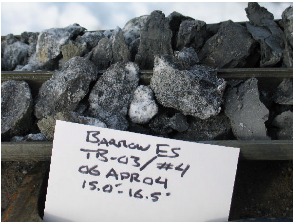
Photo 7. Example of the silt with high ice content encountered at the BIA Prospect.
