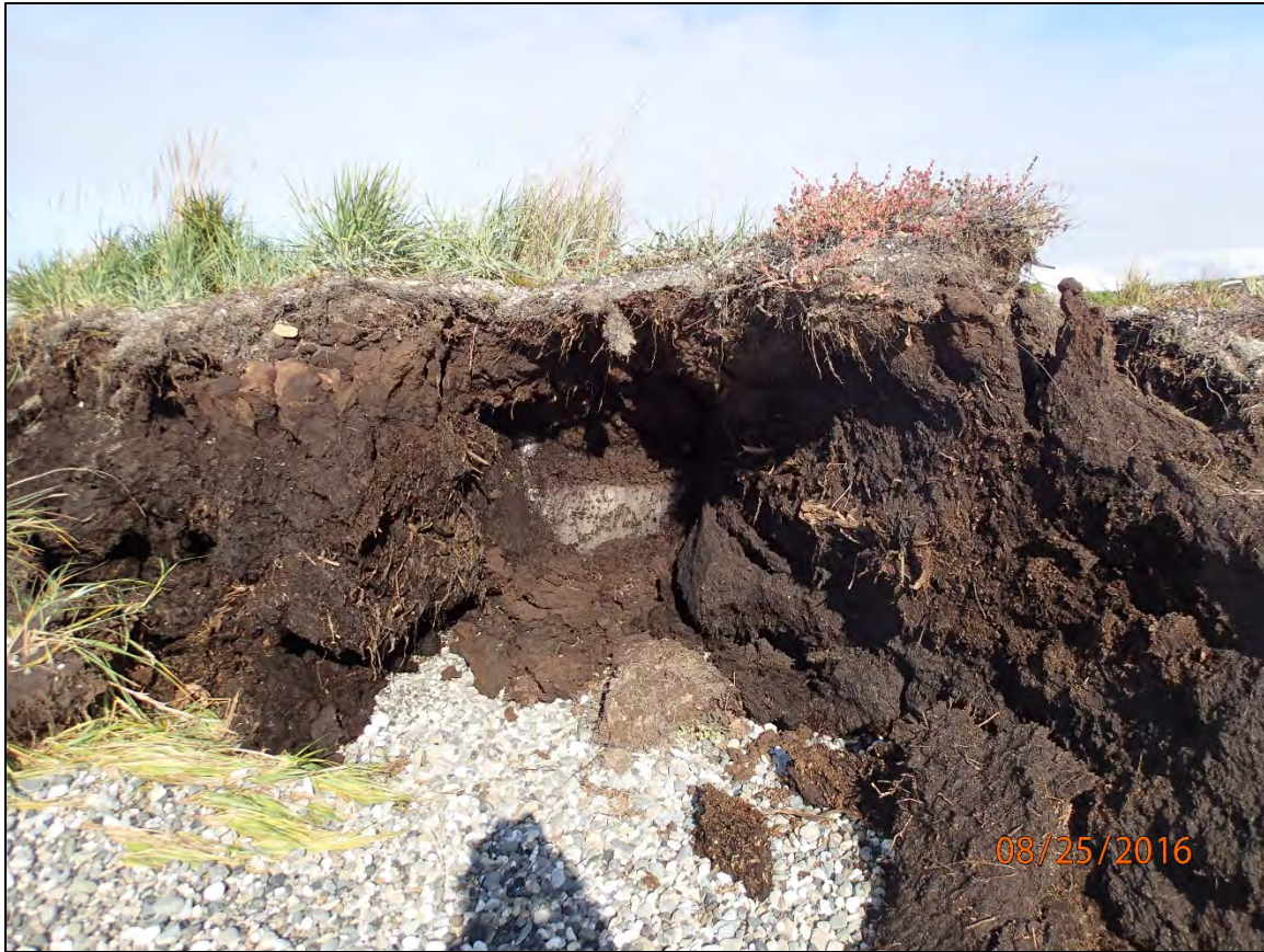
Figure 32. Exposed permafrost in the organic mat.
