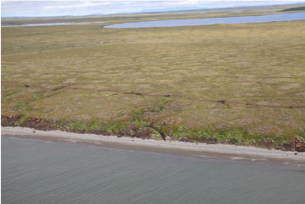
Figure 43 Reach EC - Bluffs are reduced in height and are visibly eroding (ShoreZone, n.d.)
