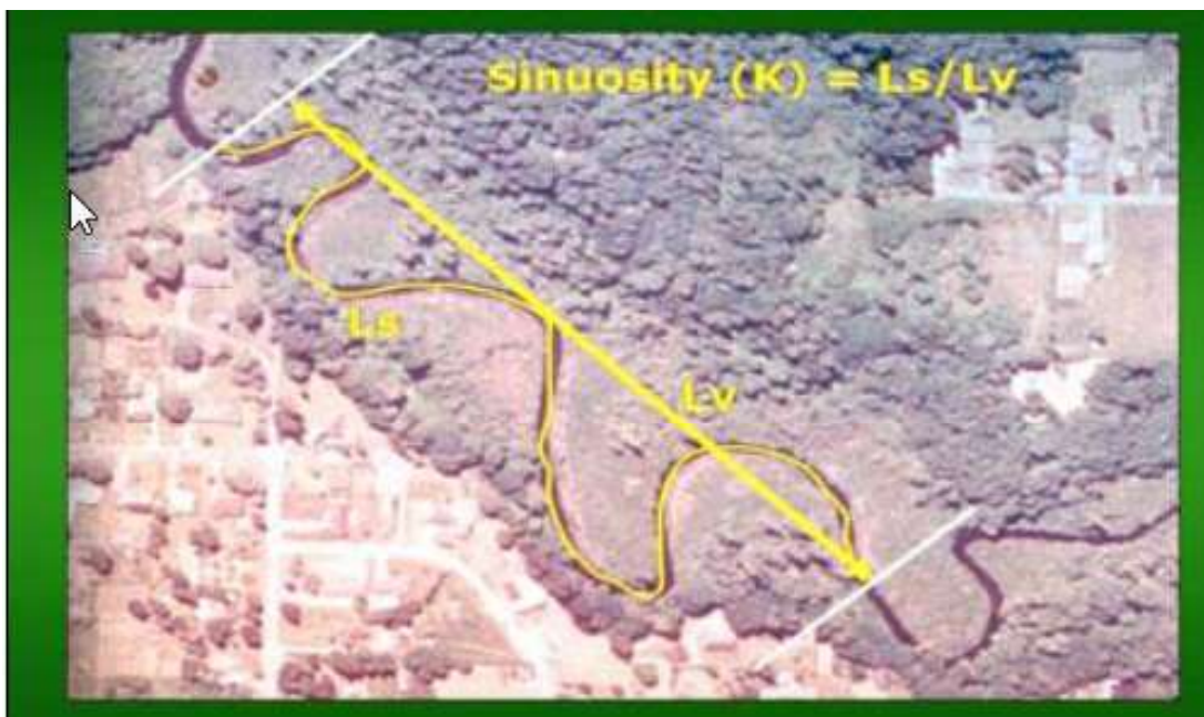
Figure 10: Sinuosity of a stream. From Rosgen (1998).
