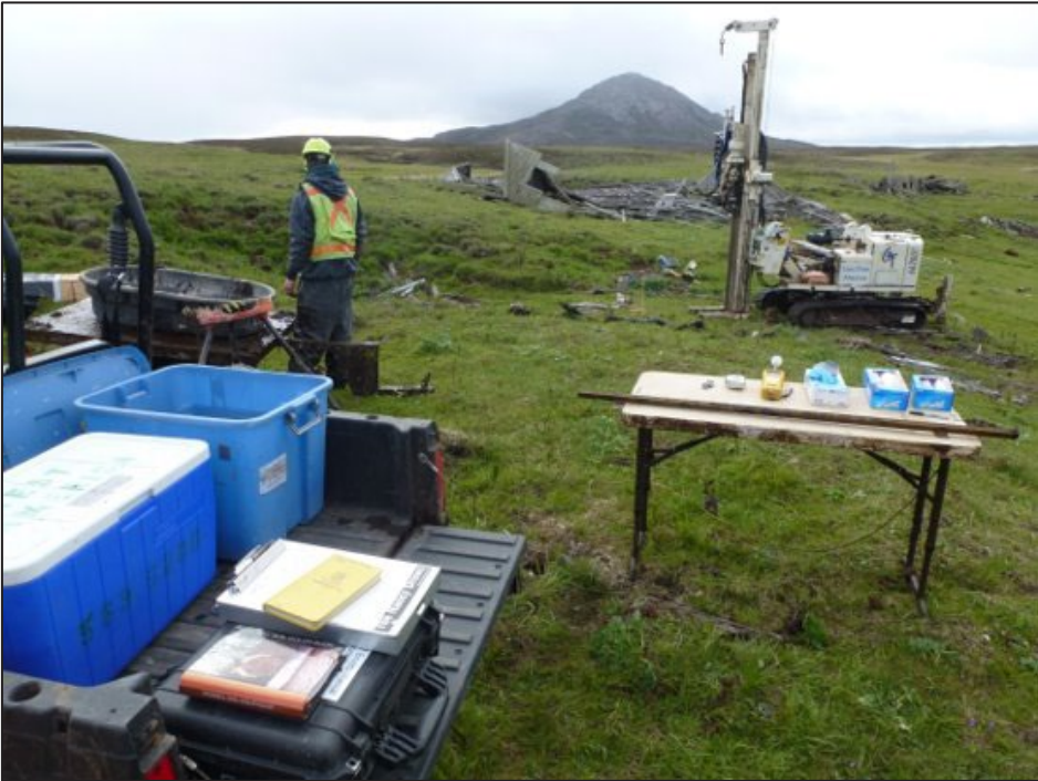
Soil sampling of a debris pile using direct push drill technology
