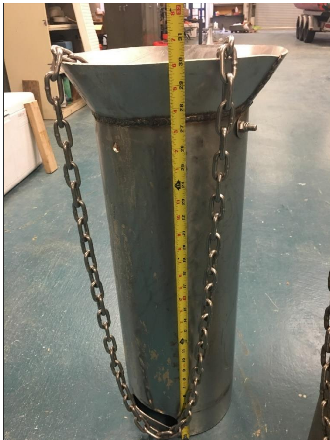
Figure 3. Barrel sampler used to collect sediments.
