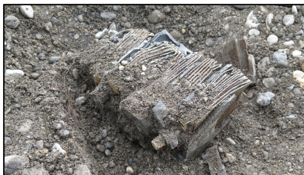
Photo 3: Exposed Lead Battery from Landfill, 2014
