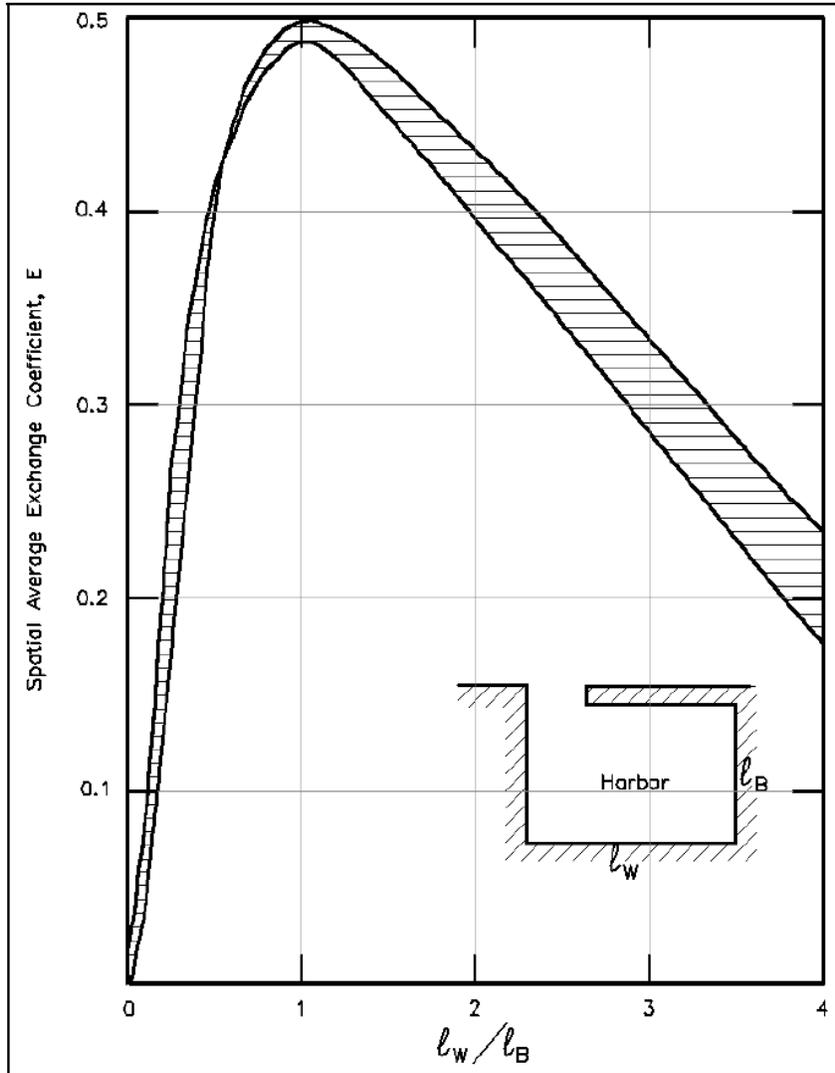
Figure 45: Exchange Coefficients – Rectangular harbor (USACE, 2008)
