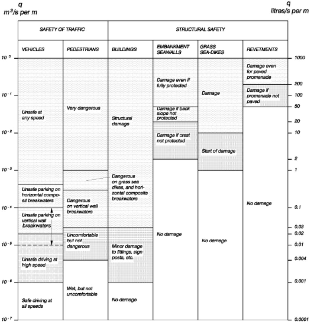
Figure 42. CEM Table VI-5-6 Critical Values of Average Overtopping Discharges (USACE, Coastal Engineering Manual, 2008).
