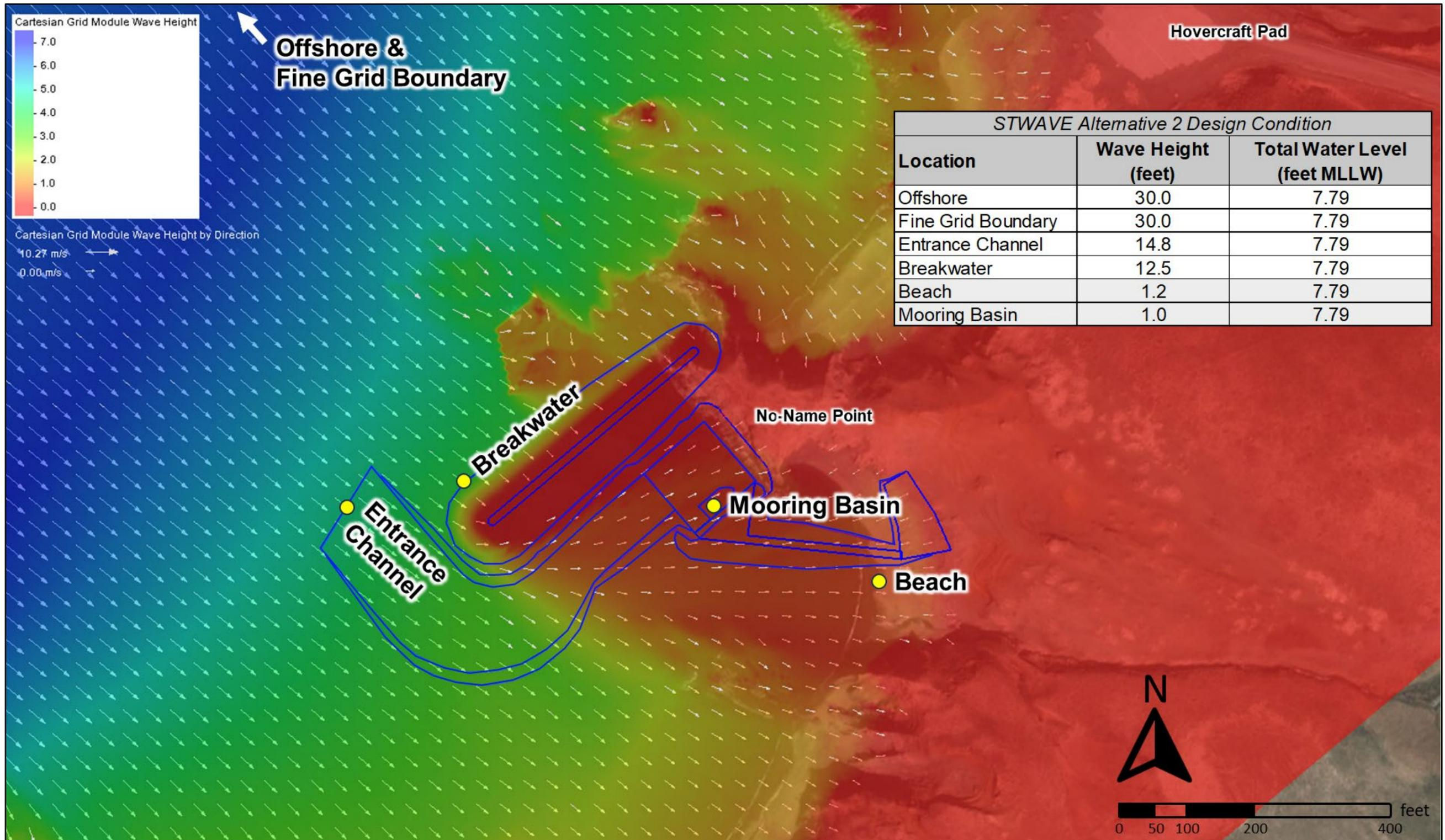
Figure 36: STWAVE Results for Alternative 2, Design Condition
