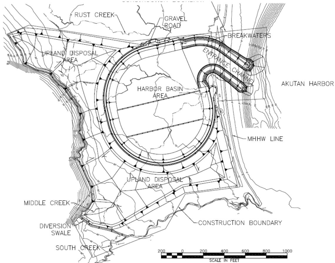
**Figure 4: Akutan Small Boat Harbor Drawing – Plan View**
