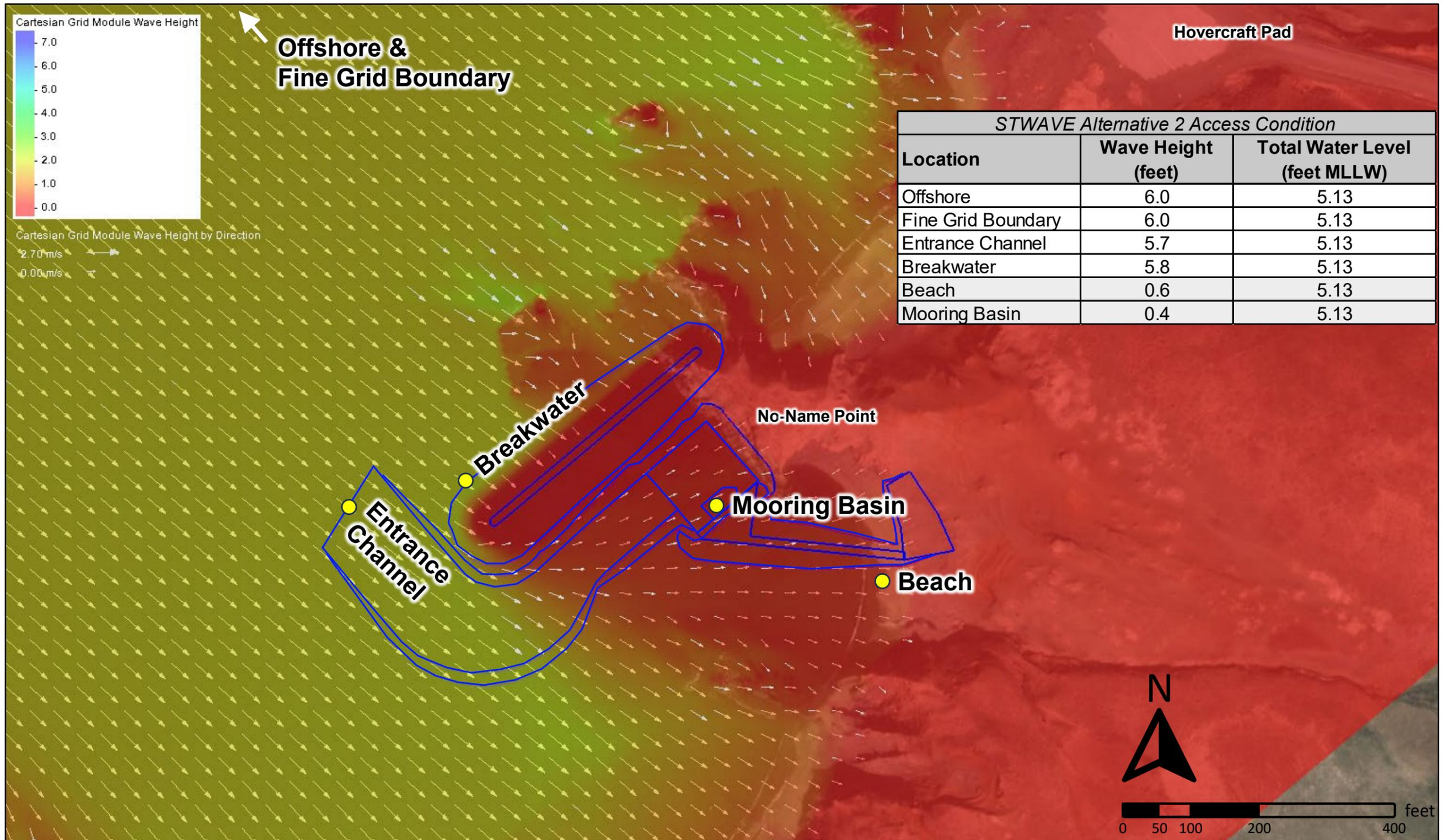
Figure 37: STWAVE Results for Alternative 2, Ferry Access Condition
