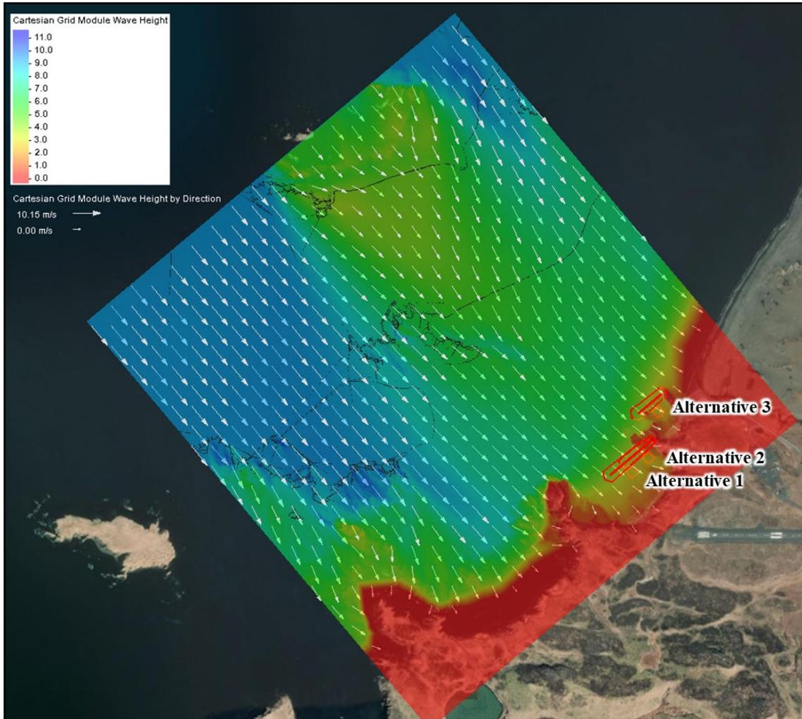
**Figure 33: STWAVE Fine Grid - Wave Height and Direction, Without Project Condition**
