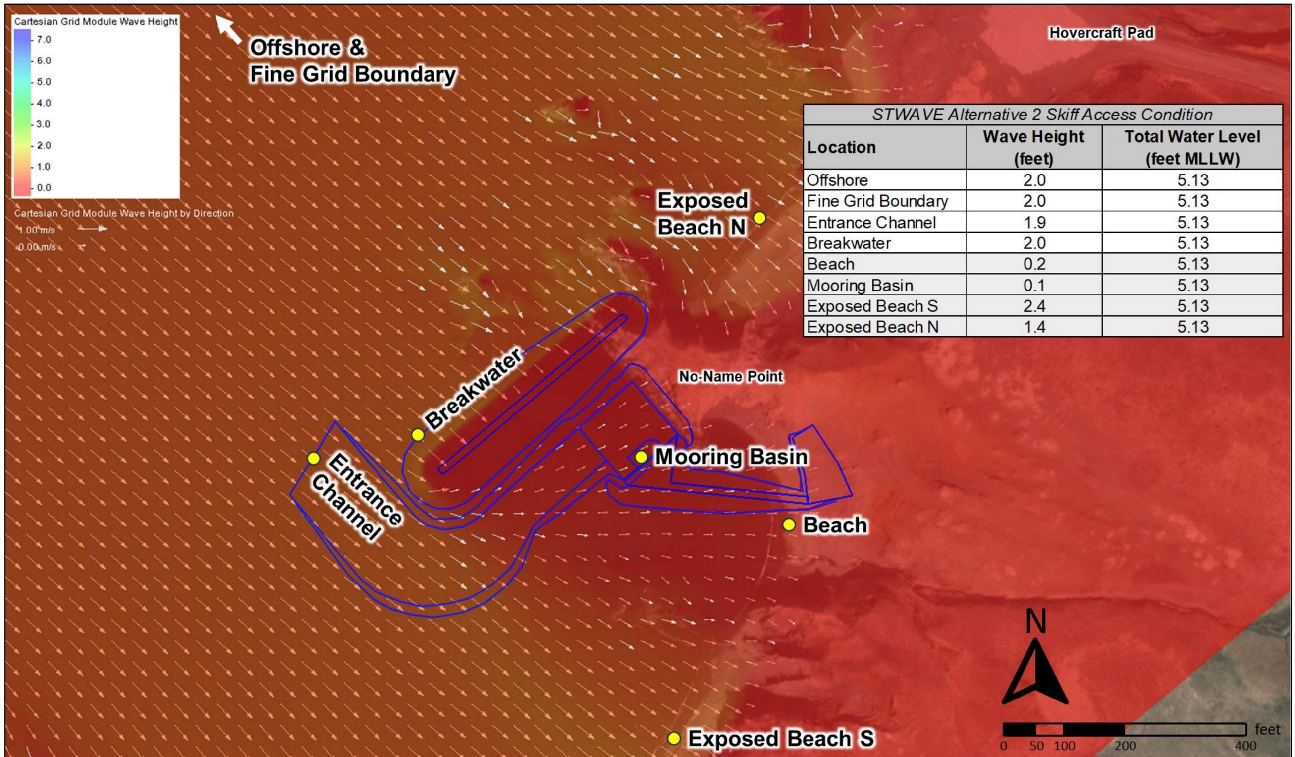
Figure 38: STWAVE Results for Alternative 2, Skiff Access Condition
