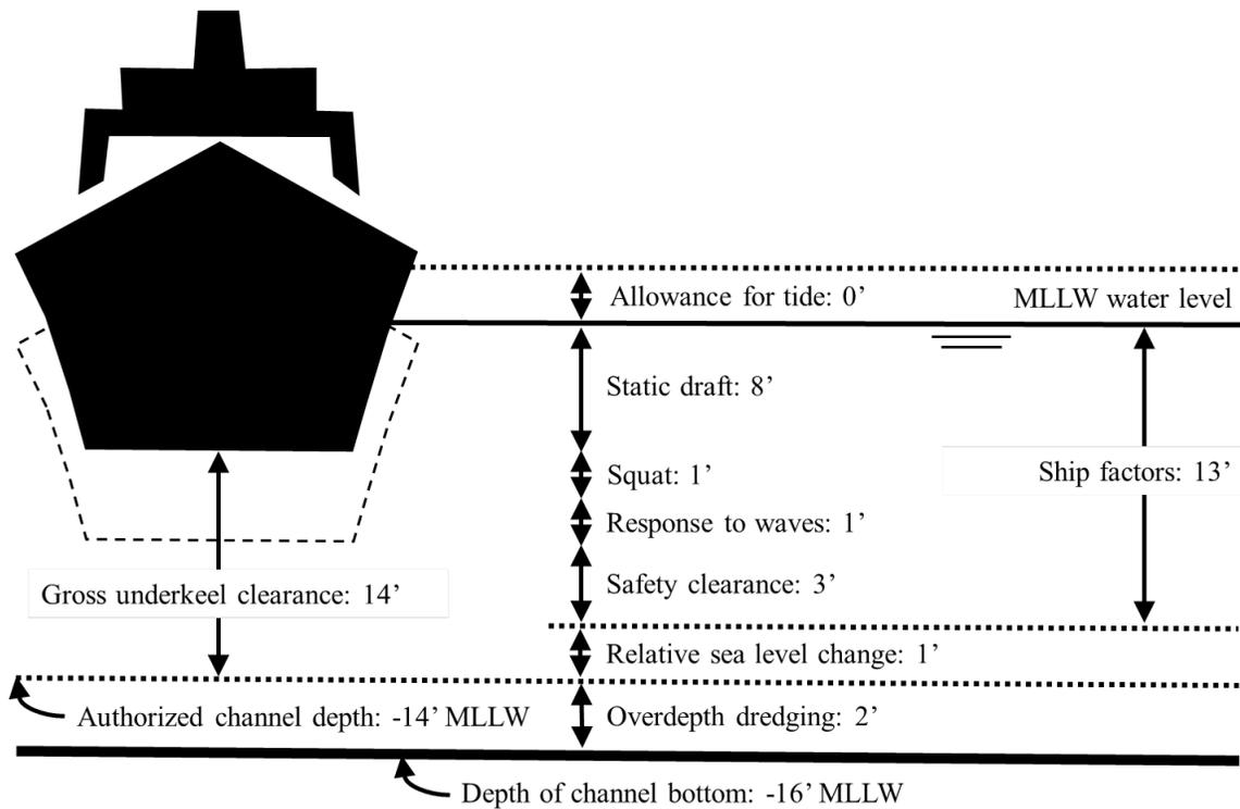
**Figure 46: Channel Design Parameters**
