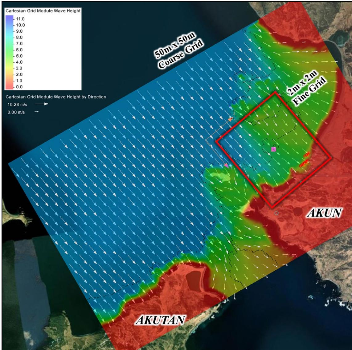
**Figure 32: STWAVE Coarse and Fine Grids - Wave Height and Direction, Without Project Condition**
