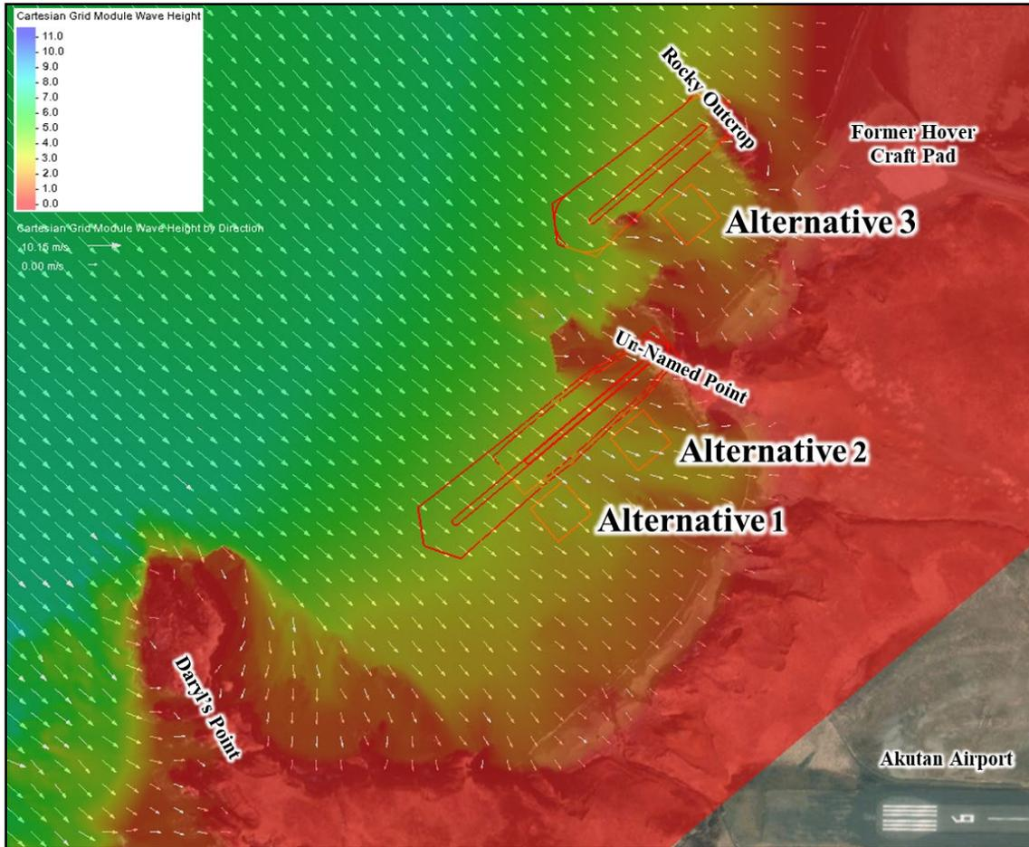
Figure 34: STWAVE Fine Grid Closeup on Alternatives - Wave Height and Direction, Without Project Condition
