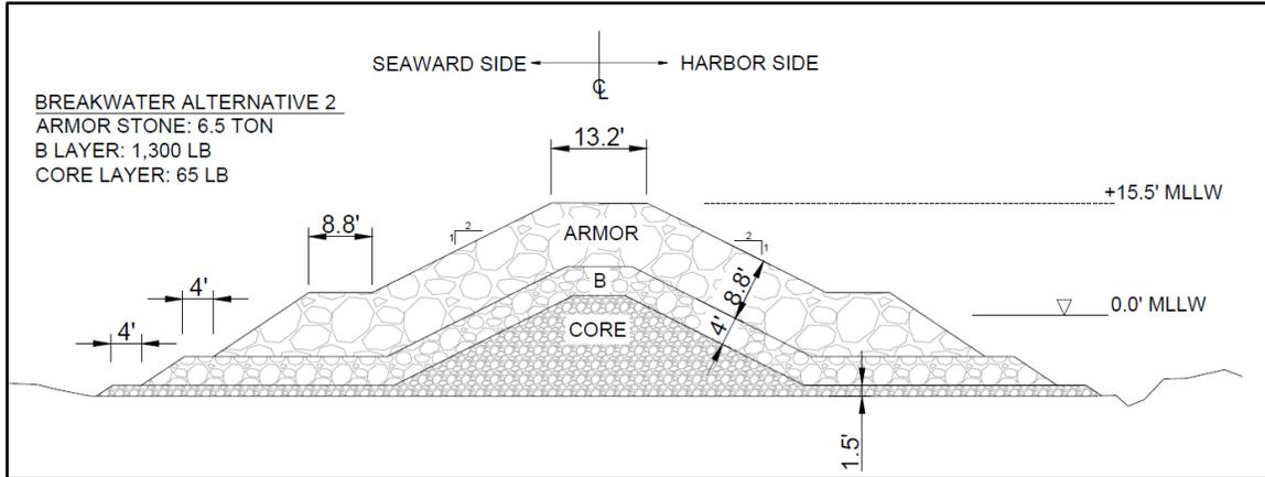
**Figure 43: Breakwater Typical Cross Section (Alternative 2)**
