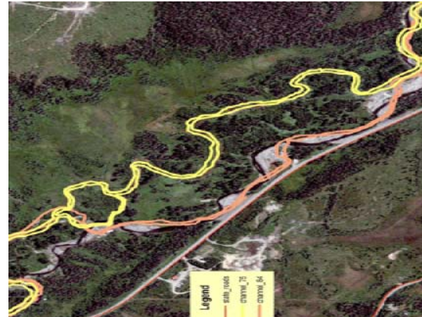
Photo 2: This photo shows the channel movement from 1975 to 1984; the channel now is very close to the Sterling Highway; aerial photo graphic courtesy of the Kenai Watershed Forum, Anchor Point Study.
