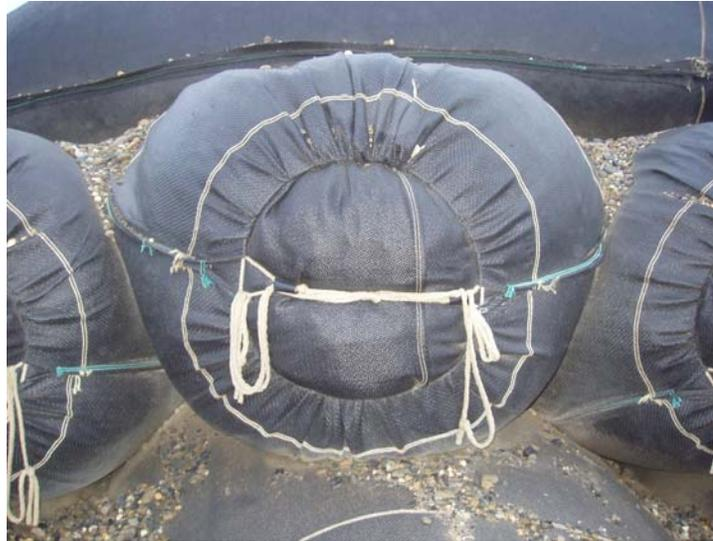
Figure 15: Photo of Engineered Sandbag Double Closure System
