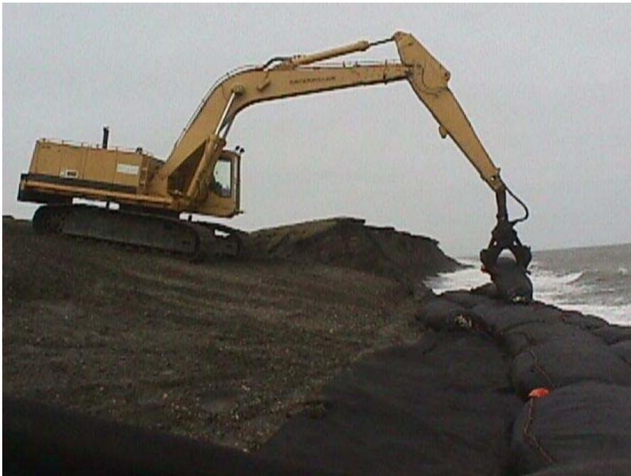
**Figure 21** Excavator with modified round half pipe over grab teeth.
