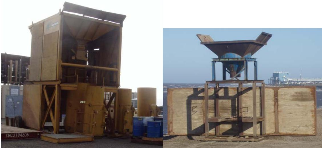
**Figure 20 Sand Bag Filling Racks.** The rack on the left is more elaborate and would allow for faster production. Loaded sandbags are normally carried inside of a large fabricated pipe with a hinging bottom lid. If the bag design includes lifted straps (preferred) they can also be lifted by the straps.
