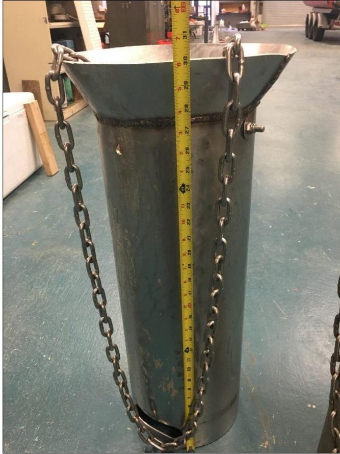
Figure 3. Barrel sampler used to collect sediments.
