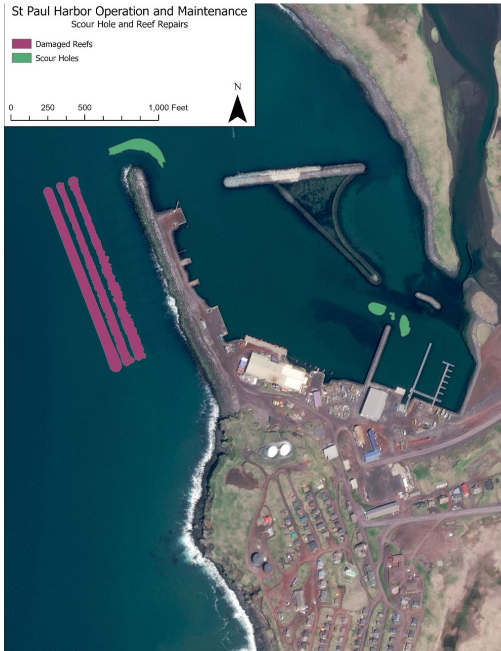
Figure 4. Saint Paul Harbor Scour Holes and Damaged Reefs
