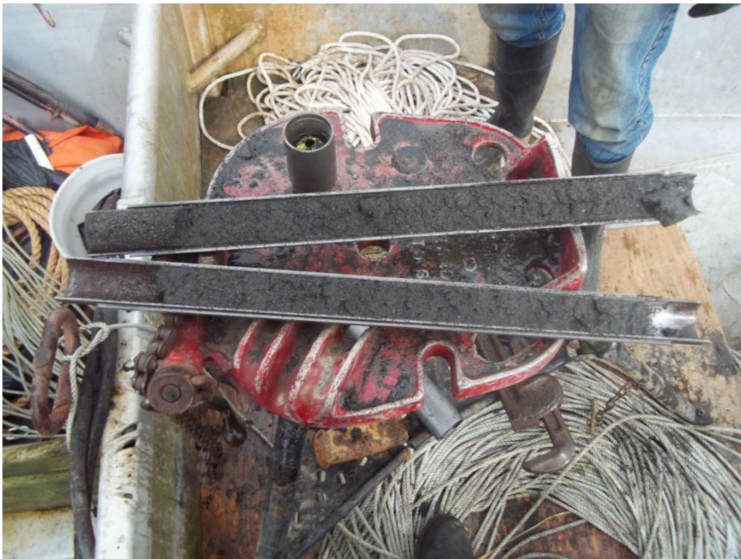
Figure 8. Split-spoon sampler with full recovery of sediment at Sediment Sampling Location 6
