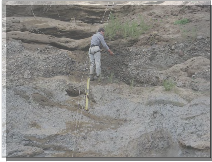
a. Cemented lag gravel (darker center bed in photo) at Soil Profile SP-C. The light gray bed below it was the dense glacial till with cobbles and boulders. There was no water observed seeping from the bluff at this location. October, 2006.
