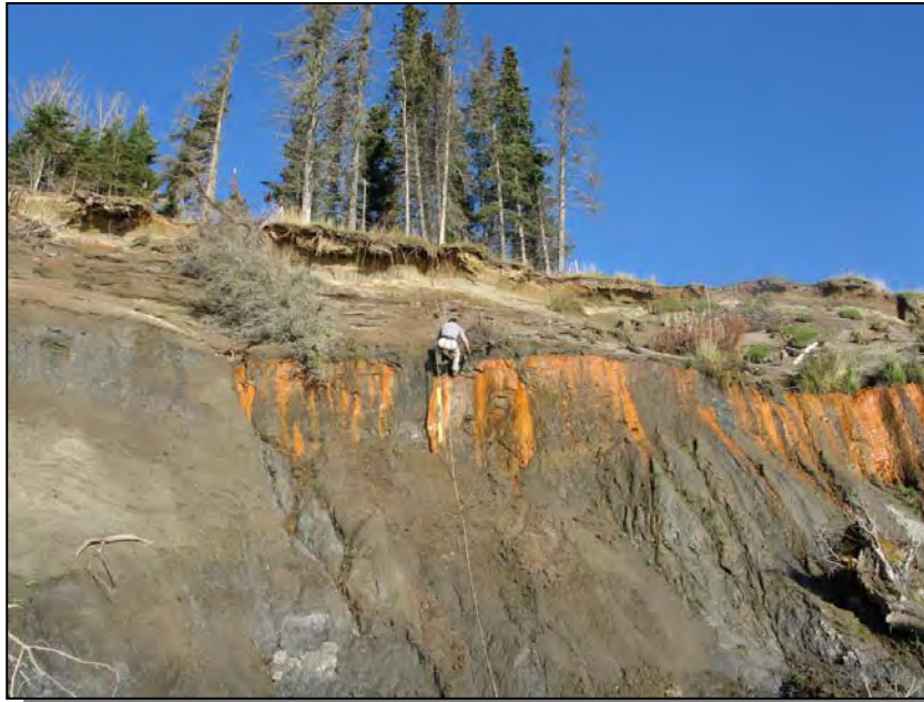
a. Rappelling down the bluff face at Soil Profile SP-D. The four-foot yellow electronic level was used to measure slope angle. Slope distances were measured using the white tape. October, 2006.
