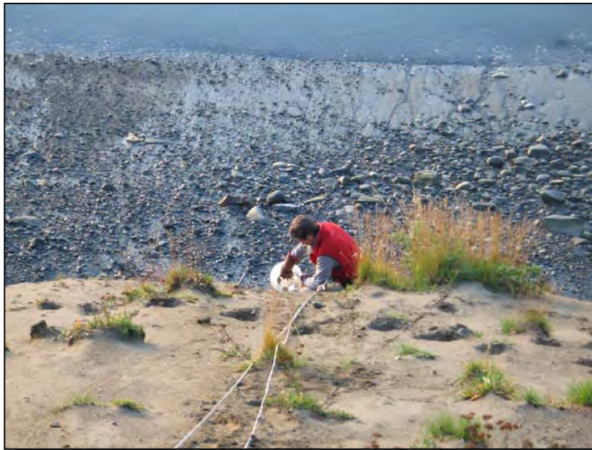
b. Measuring water flow from the bluff at Soil Profile SP-E. The procedure involved catching the flow and then measuring in a bucket. October, 2006.
