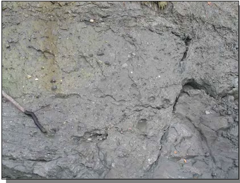
b. Scattered gravel in clayey glacial till. Much of this gravel may be “dropstones” derived from floating glacial ice. October, 2006.
