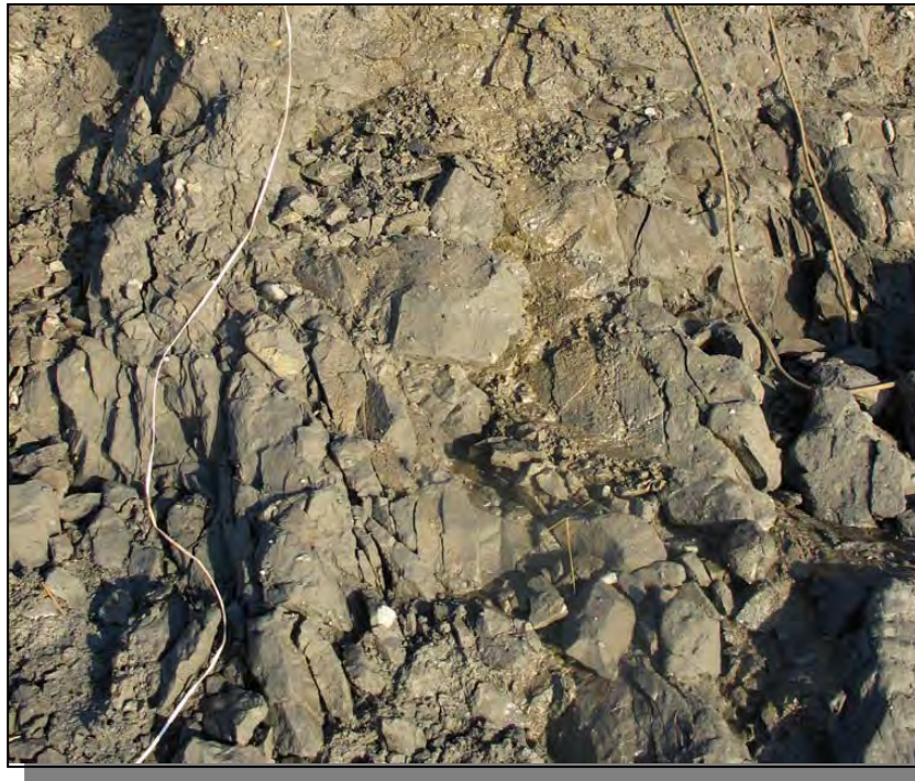
b. Glacial till exposed at the bottom of the bluff. Note the bedrock-like jointed appearance of the clay. October, 2006.
