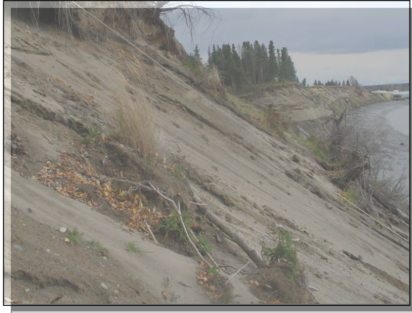
a. Slope in alluvial unit at Soil Profile SP-F. Overhanging surficial soil layer can be seen at upper left. October, 2006.
