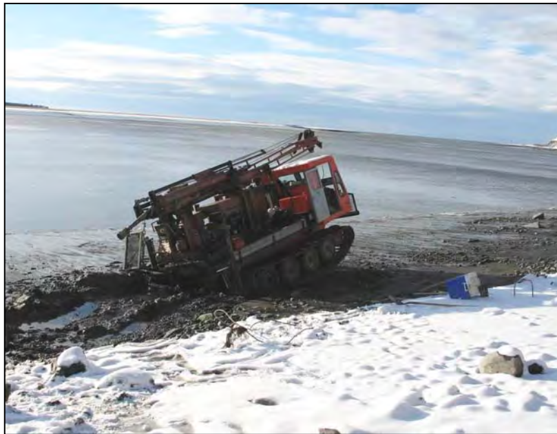
b. The Nodwell has sunk into unfrozen mud below the high tide line (edge of snow covered area). The surface of the mud was frozen under the snow covered area. November 10, 2006.
