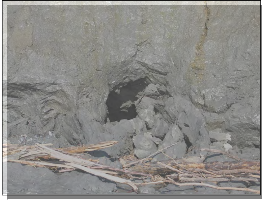
a. Caves formed in bluff by erosion of sand pockets. Note caving of clay caused by undermining due to removal of sand. October, 2006.
