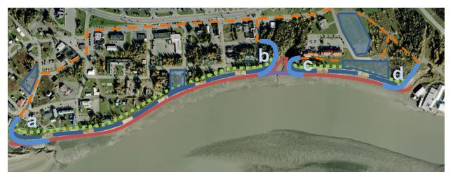
**Figure F-7. Fill Zones in Plan View**
