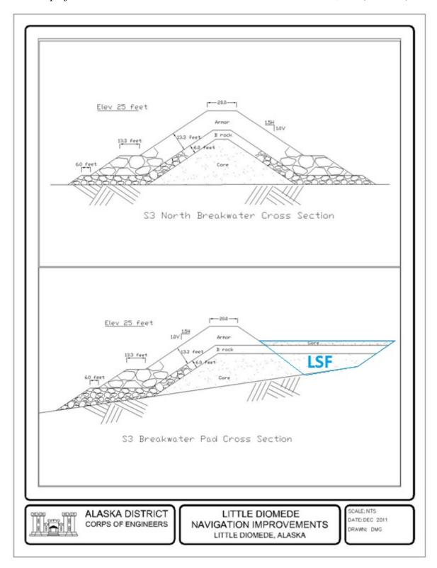
Figure 9. Typical Cross-section of Southern Breakwater LSF
