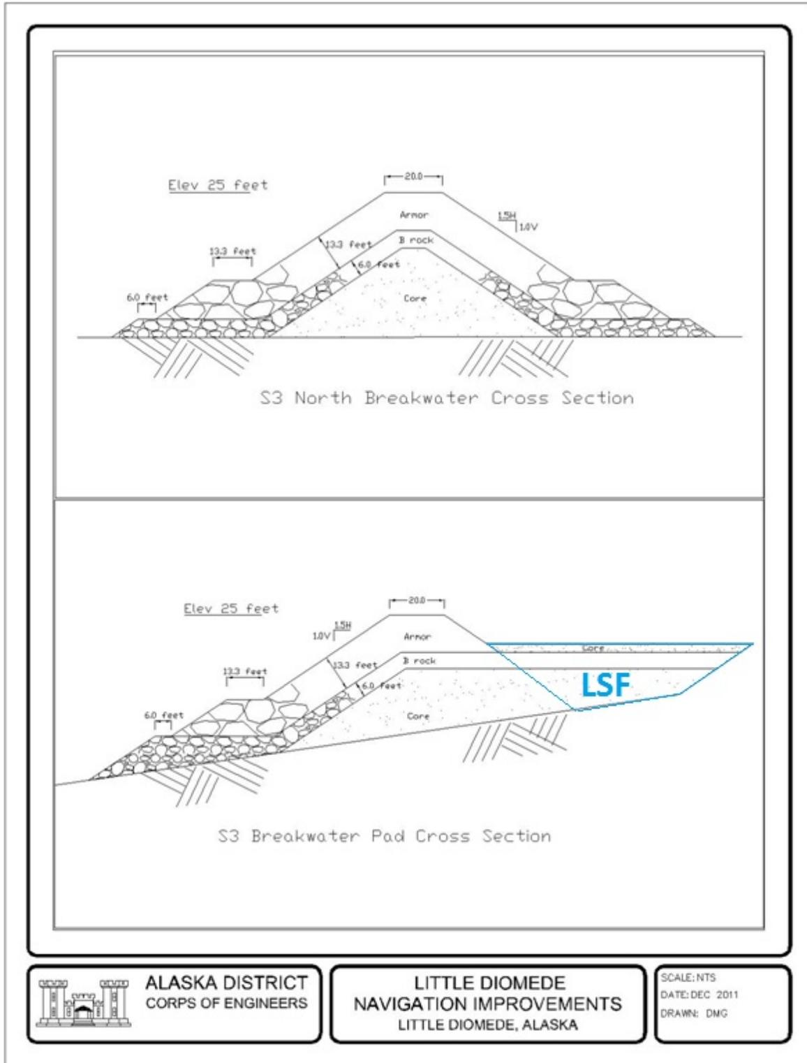
Figure 9. Typical Cross-section of Southern Breakwater LSF
