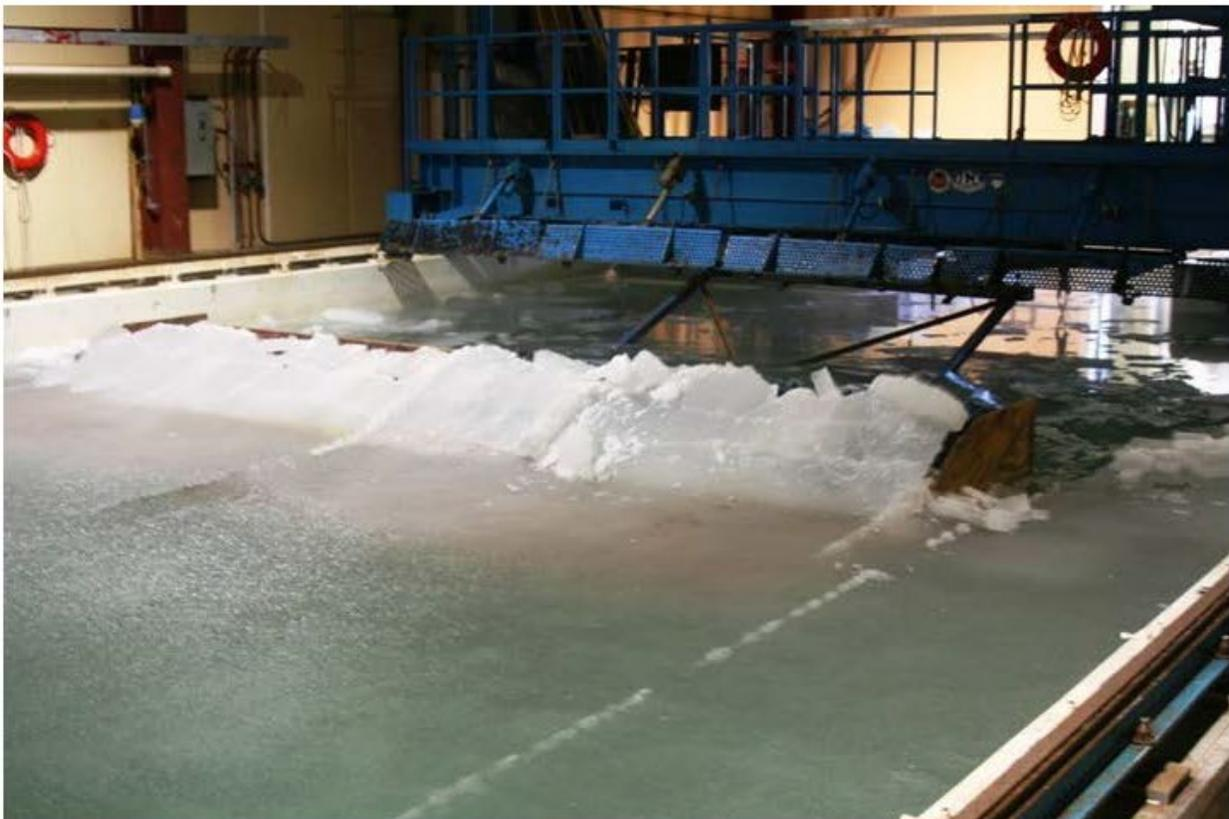
**Figure 109. Revetment Test Section being Pushed by Carriage**
