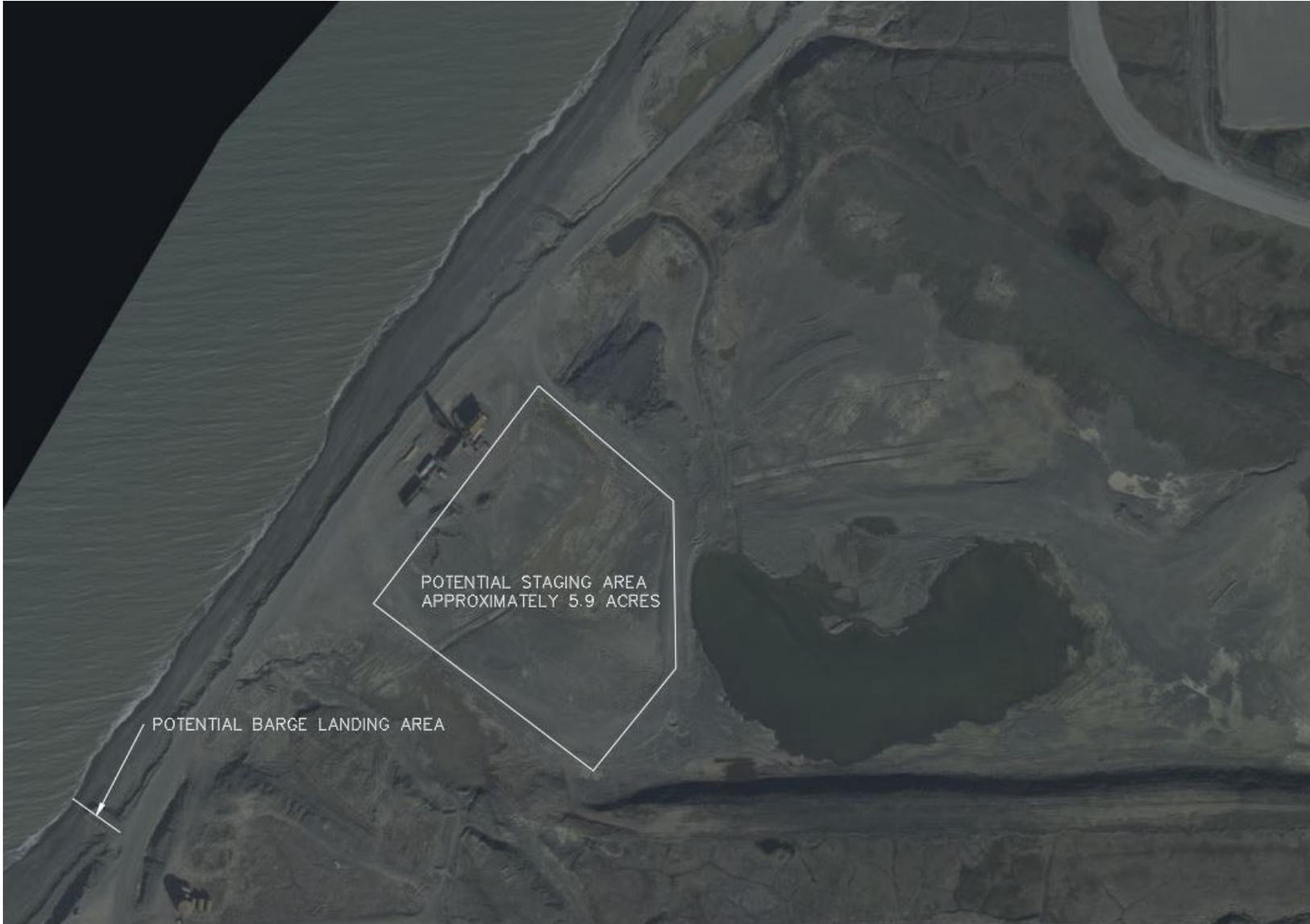
**Figure 117. Potential Staging Area and Barge Landing at State of Alaska DOT Borrow Pit**
