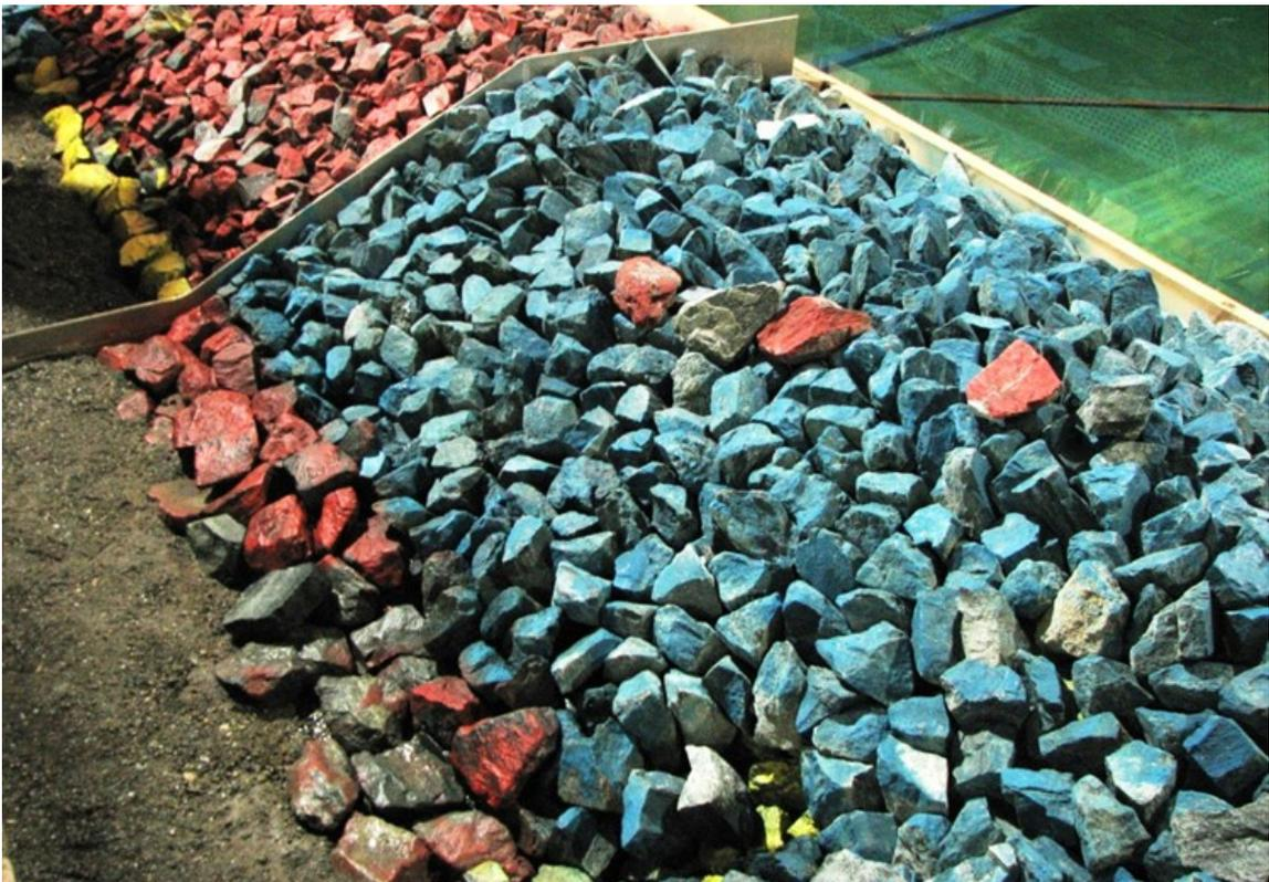
**Figure 112. Rock Revetment after Ivu Event Testing, some Toe Rock Moved during Test, but the Revetment Slope Stayed Intact. 8-ton Armor Rock (Blue Slope) with 13-ton Toe Rock (Red Toe)**
