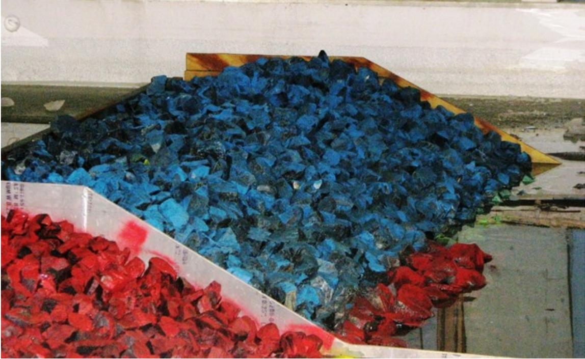
**Figure 111. Revetment before Testing. 8-ton Armor Rock (Blue Slope) with 13-ton Toe Rock (Red Toe)**
