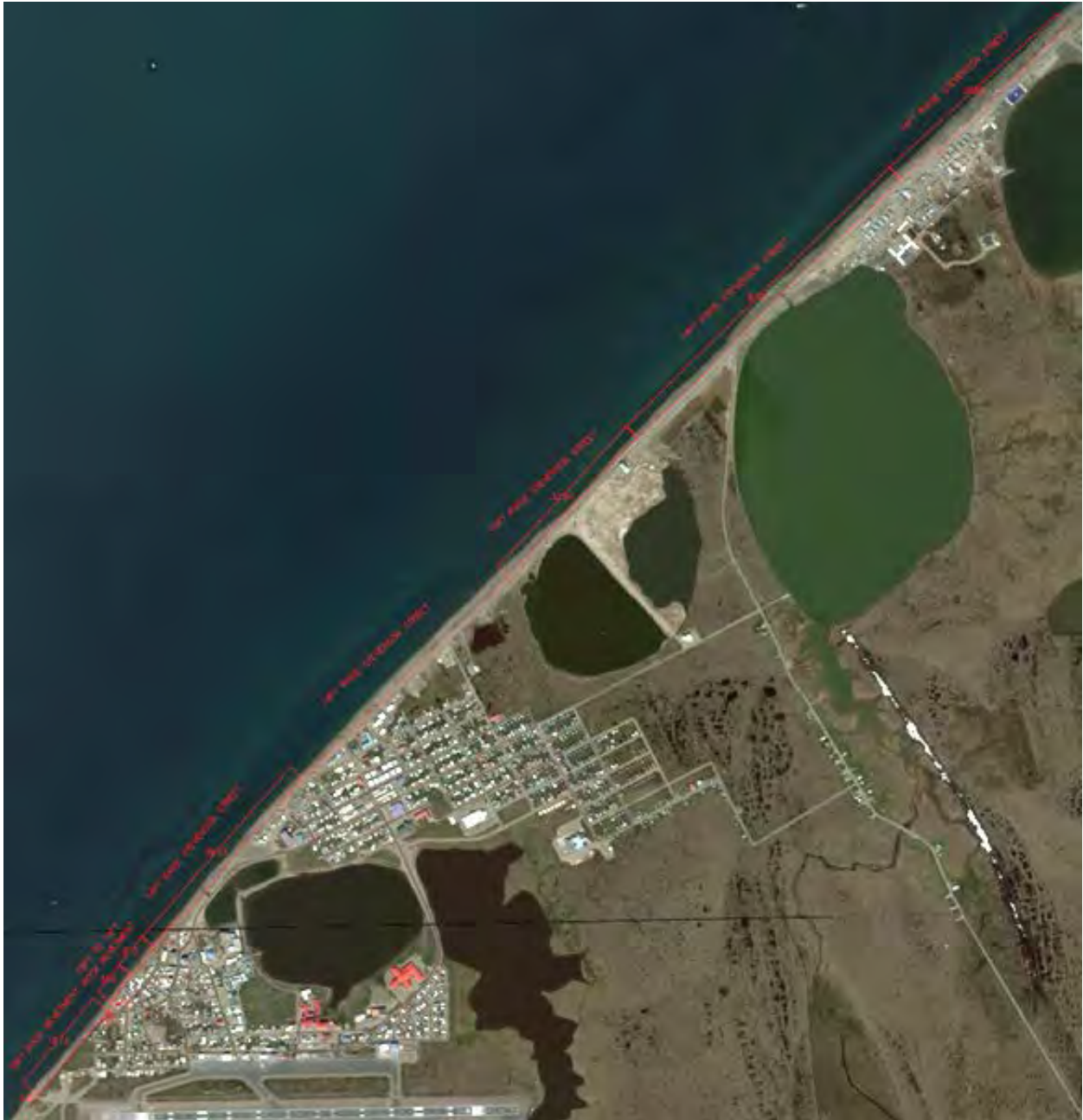
Figure 119. Alternative 2b: Rock Revetment at Bluff and Raise Stevenson Street.
