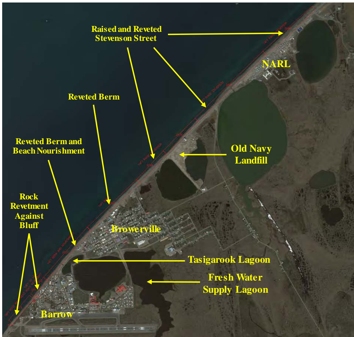
Figure 3 - Alternative 6A (Combination Rock Revetment, Raised Stevenson Street, Revetted Berm, and Beach Nourishment).
