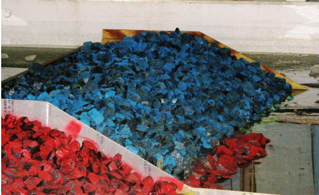
Figure 109. 8-Ton Armor Stone (Blue Slope) with 13 Ton Toe (Red Toe Stone) Revetment Before Ice Testing.
