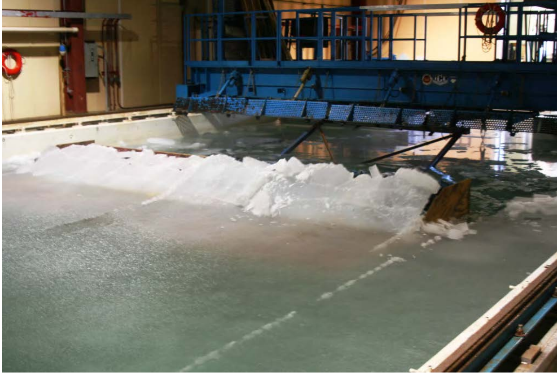
Figure 107. Revetment Test Section Being Pushed by Carriage.
