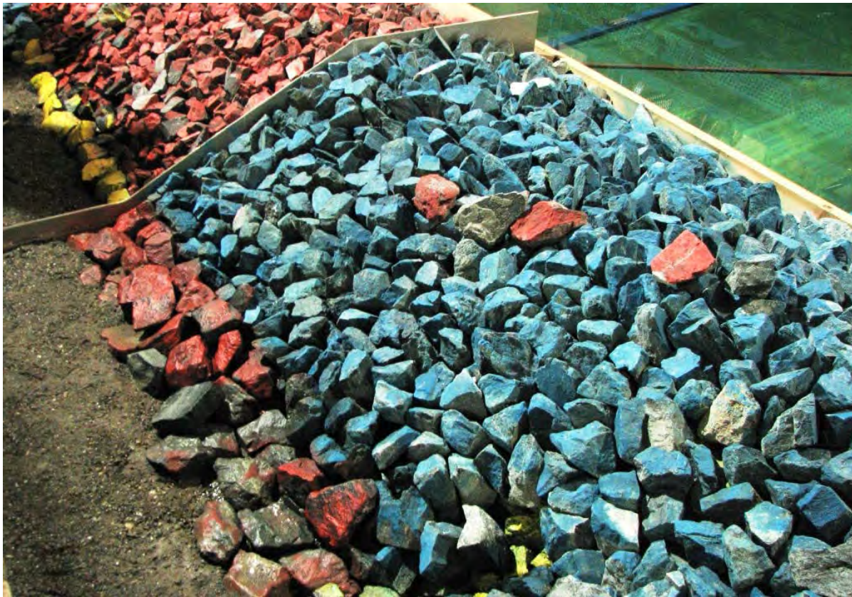
Figure 110. 8-Ton Armor Stone (Blue Slope) with 13 Ton Toe (Red Toe) Stone Revetment After Ice Testing. Some Toe Stone Moved During Test, But The Revetment Slope Stayed Intact.
