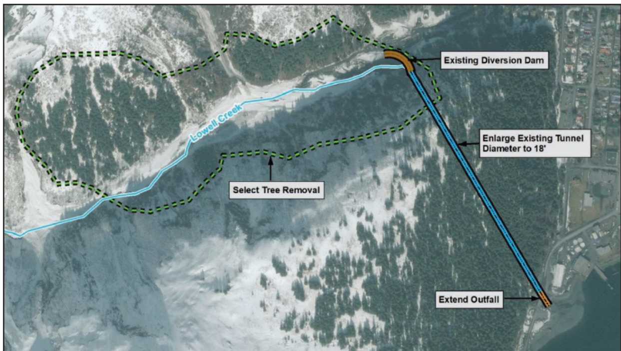
Figure 23. Alternative 3A: Enlarge Current System to Convey Larger Flow with 18-ft-Diameter Tunnel.
