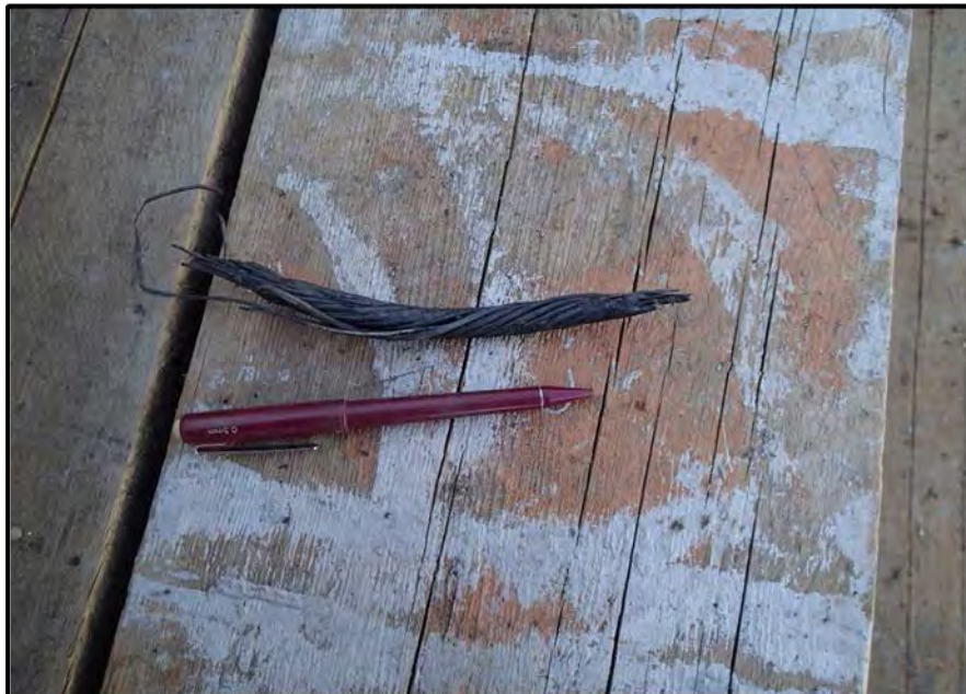
Figure 3. Part of the cable that was caught in the anchor of the landing craft RB.
