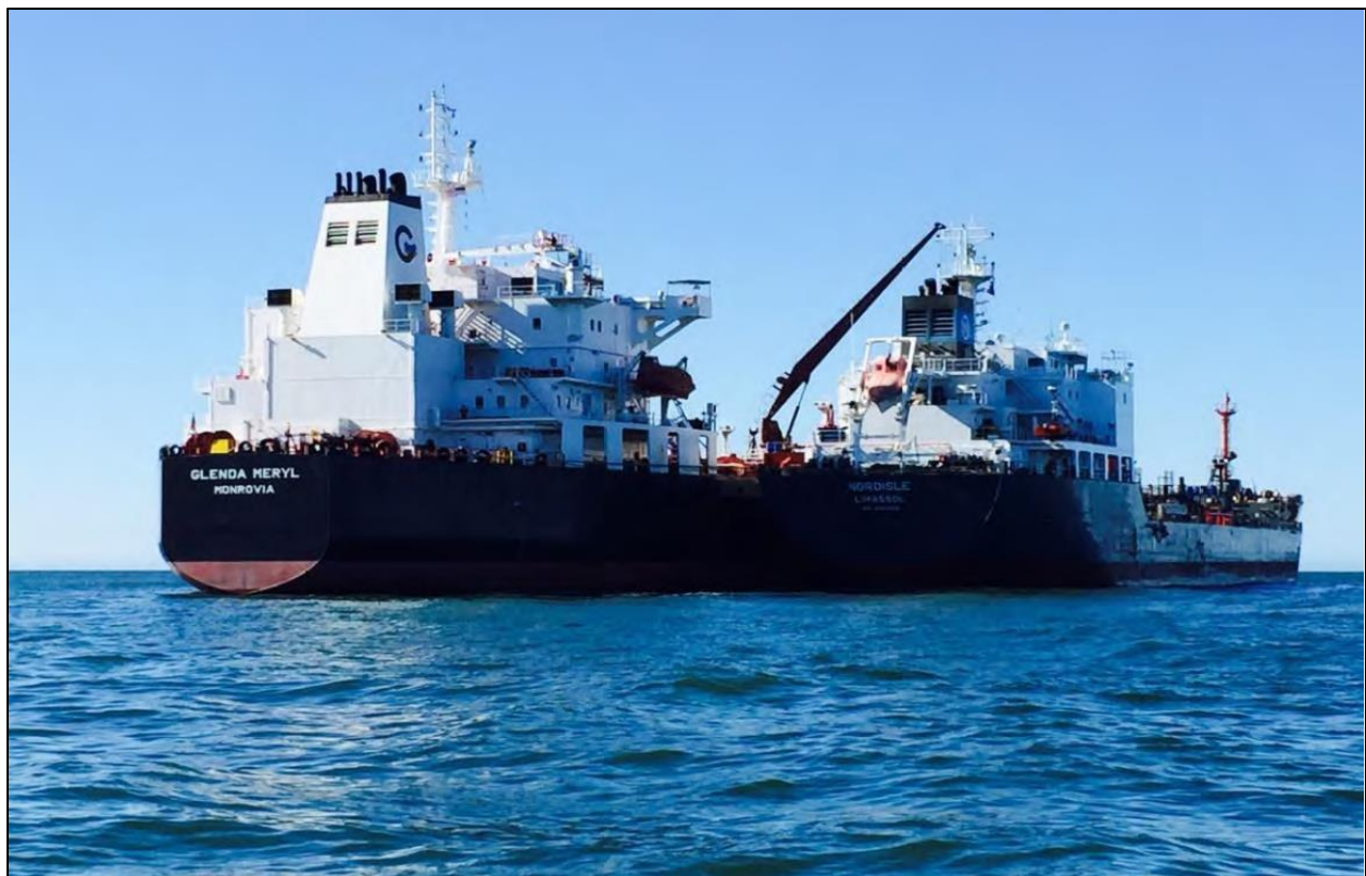
Figure 24 MR Tanker lightering to smaller “pocket” tanker offshore of Nome
