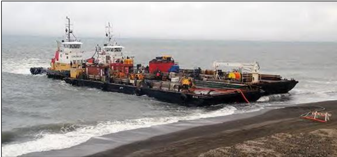
Figure 21. Fuel lighter delivering fuel over the shore via hose connection
