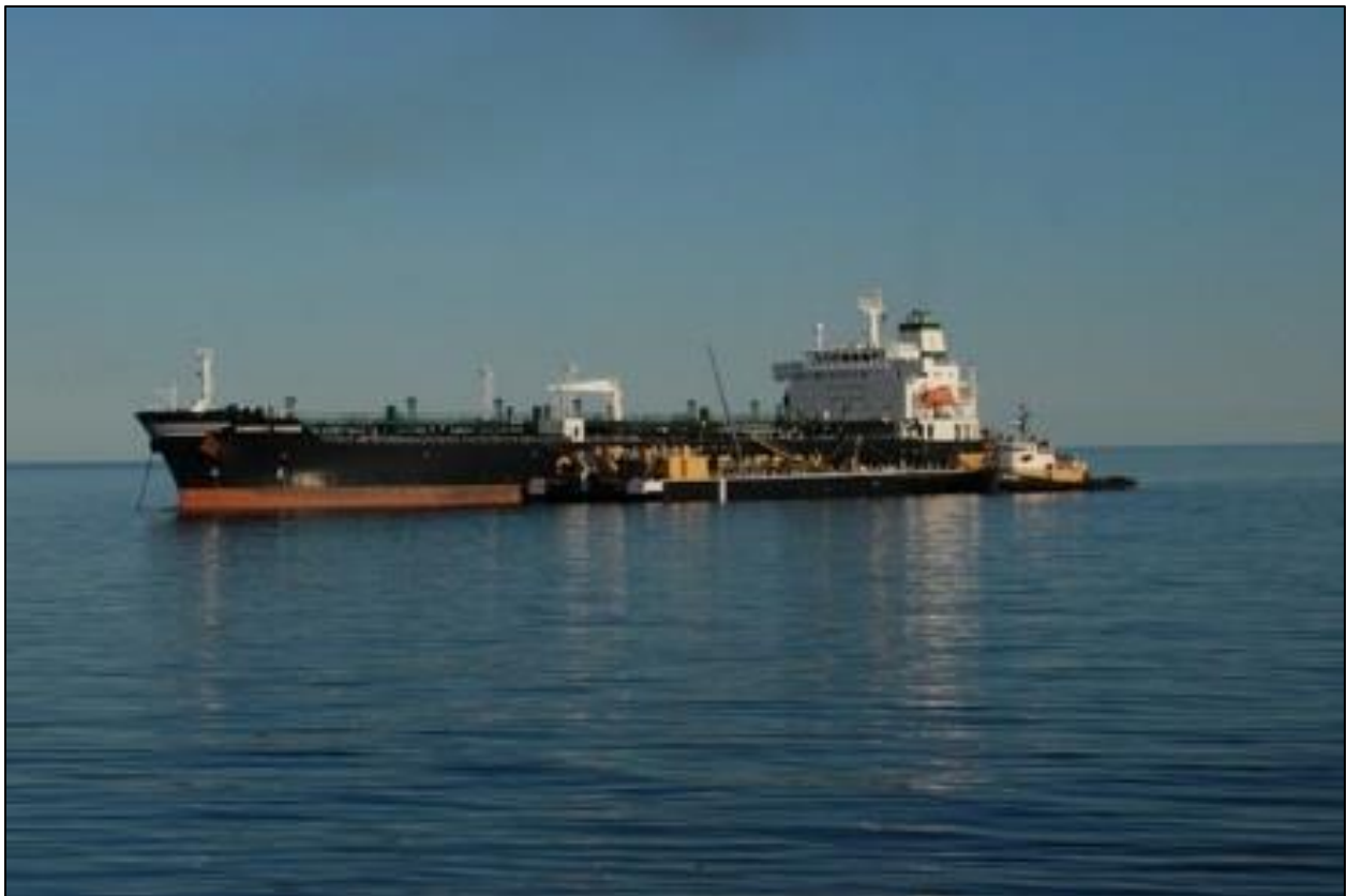
Figure 23. MR Tanker lightering to small local delivery barge
