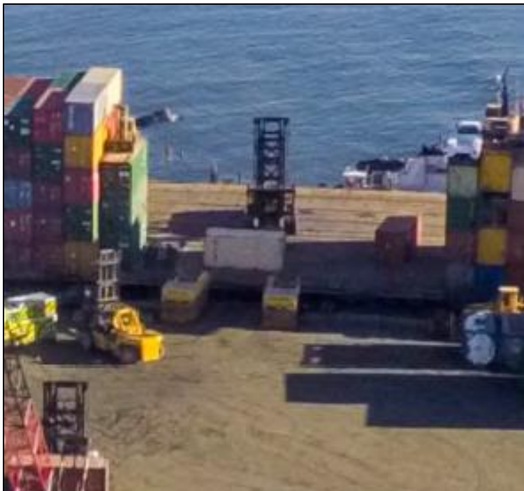
Figure 10. Forklifts using “pass-pass” technique to unload cargo containers
