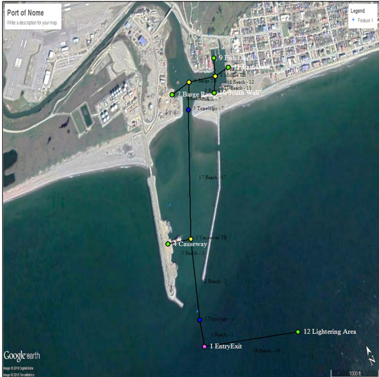
Figure 42. Port of Nome HarborSym network for Future without Project Condition
