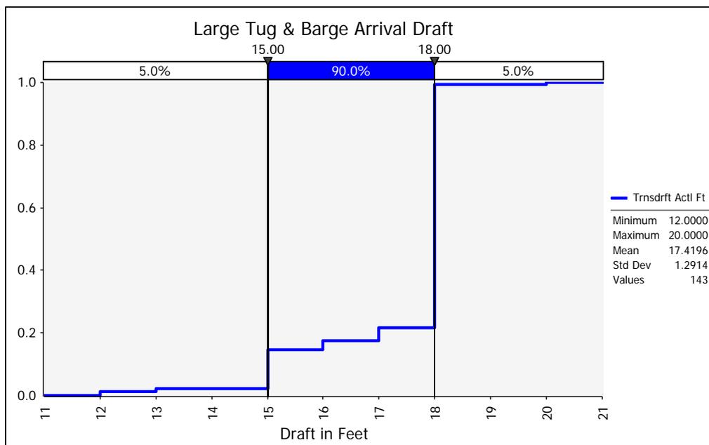
Figure 19. Figure 19 CDF for Large Tug & Barge combos Arrival Drafts into Nome 2003-2017
