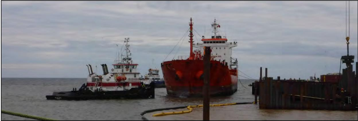
Figure 14. Private tugs assisting chartered tanker in docking at Causeway
