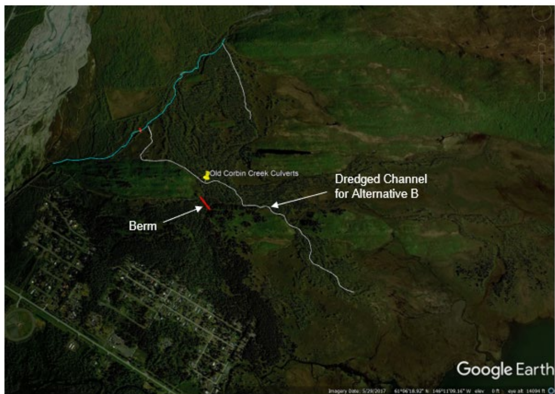
Figure 15. Full extent view of the 1.5-mile-long dredged channel on Old Corbin Creek for Alternative B.
