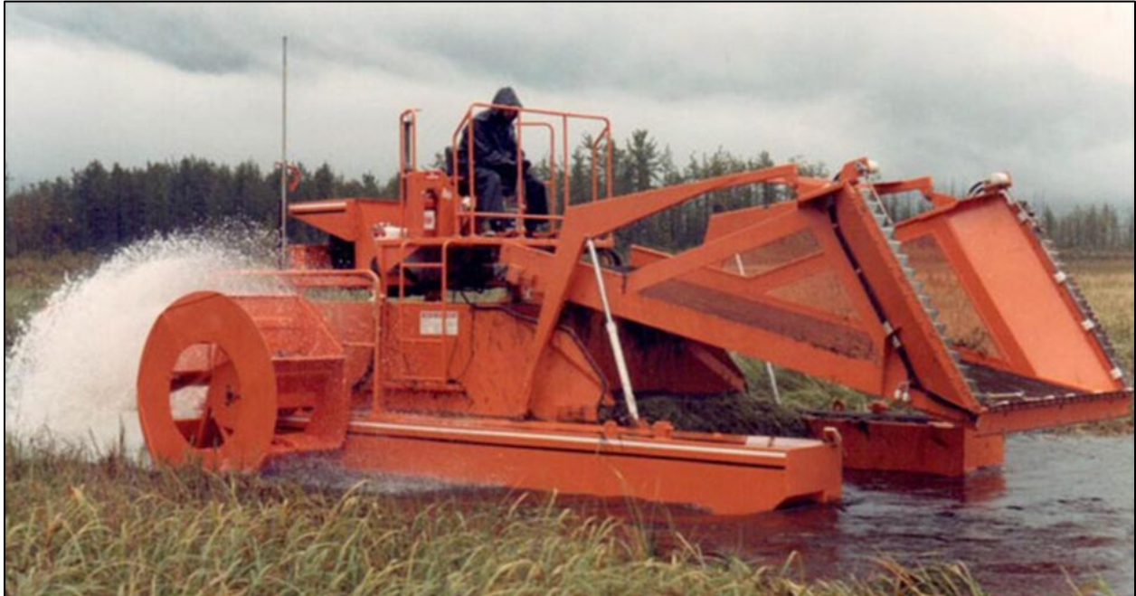
Figure 4. Mechanical weed harvesting of macrophytes at Robe Lake by VFDA.
