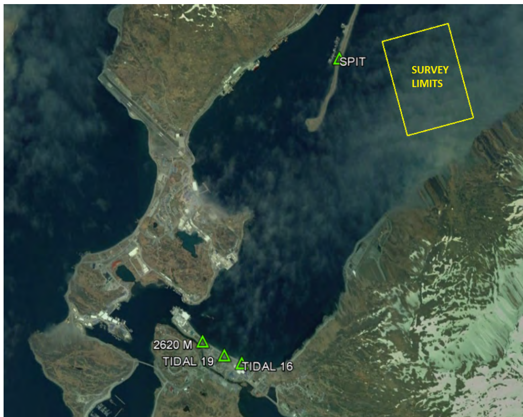
Figure 23 Semi-Permanent RTK Base Station "SPIT" established near project area
