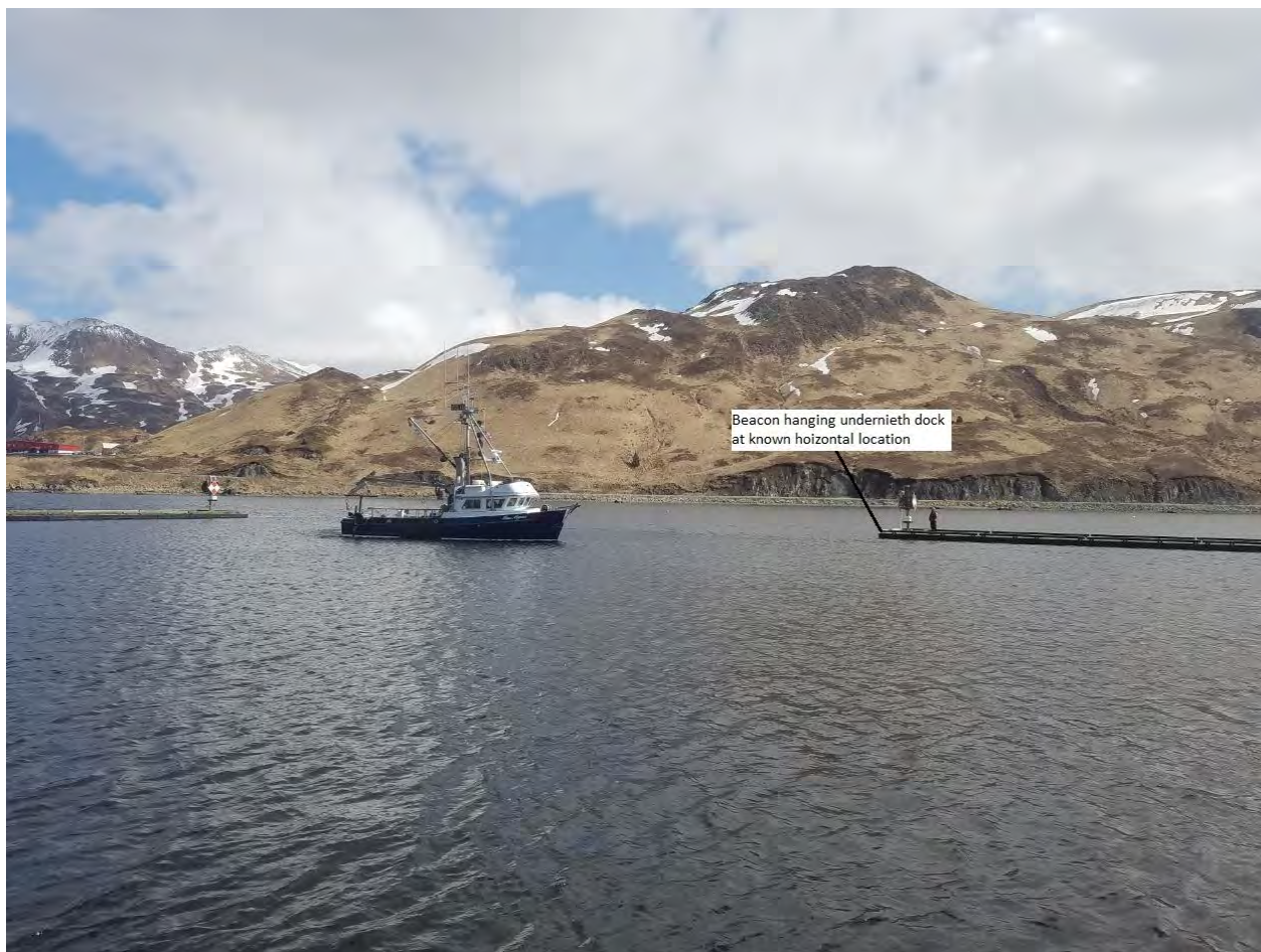
Figure 26 Vessel performing USBL Calibration
