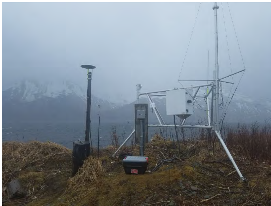
Figure 24 Semi-Permanent RTK Base Station "SPIT" GNSS & VHF Antennas installed at weather station
