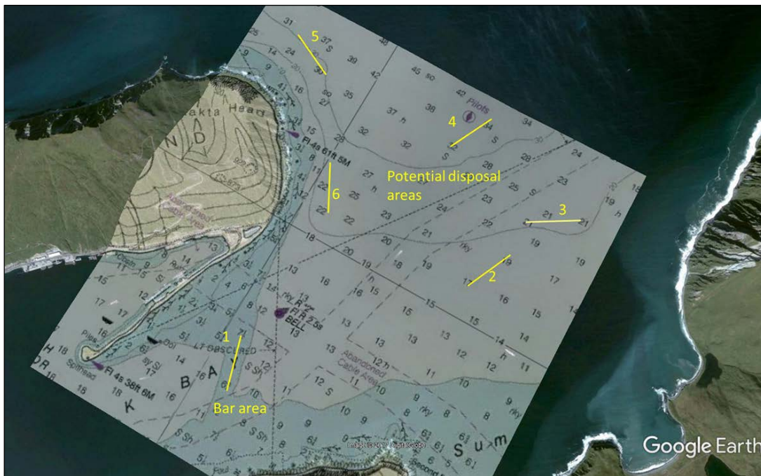
Figure 6. Potential Dredged Material Placement Areas
