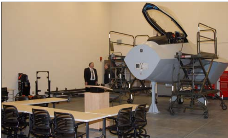
An F-22 seat and canopy trainer in the 372nd Training Squadron, Detachment 14, facility also will serve as the fire department's place to practice emergency pilot extraction. (Below) Fully-automated classrooms are capable of handling new digital training materials with graphics-intensive coursework. (Photos by Curt Biberdorf)
