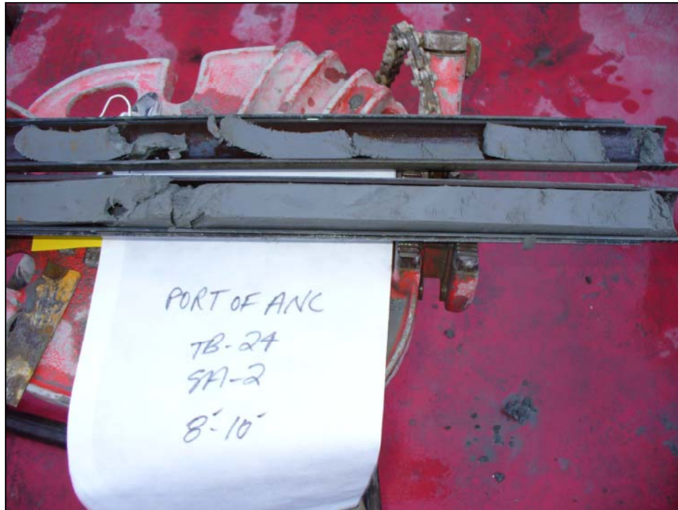
Photograph 6: Sample from test boring AP-4606 taken between 8.0 and 10.0 feet below the mudline.
