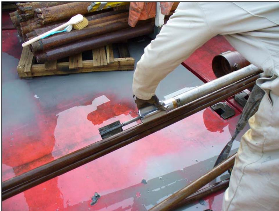
Photograph 2: View of 55-millimeter x 110-millimeter rectangular vane used during the field vane shear testing.
