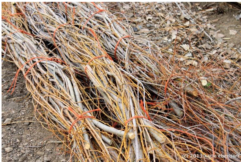
Photo 19: Live Fascine Bundles Prior to Installation
