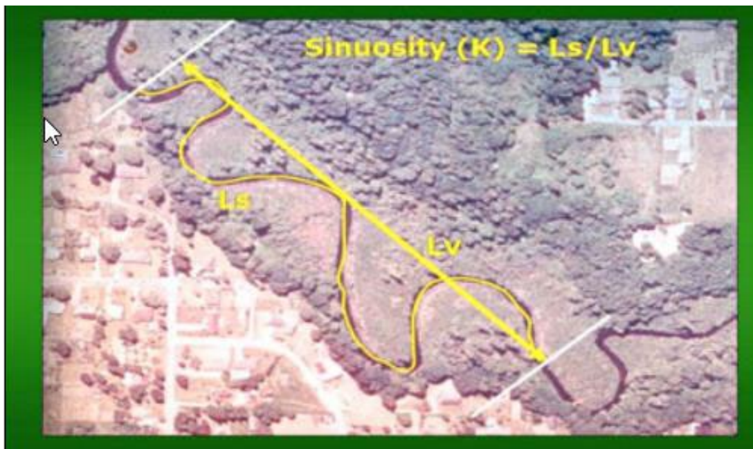
Figure 9: Sinuosity of a stream. From Rosgen (1998).
